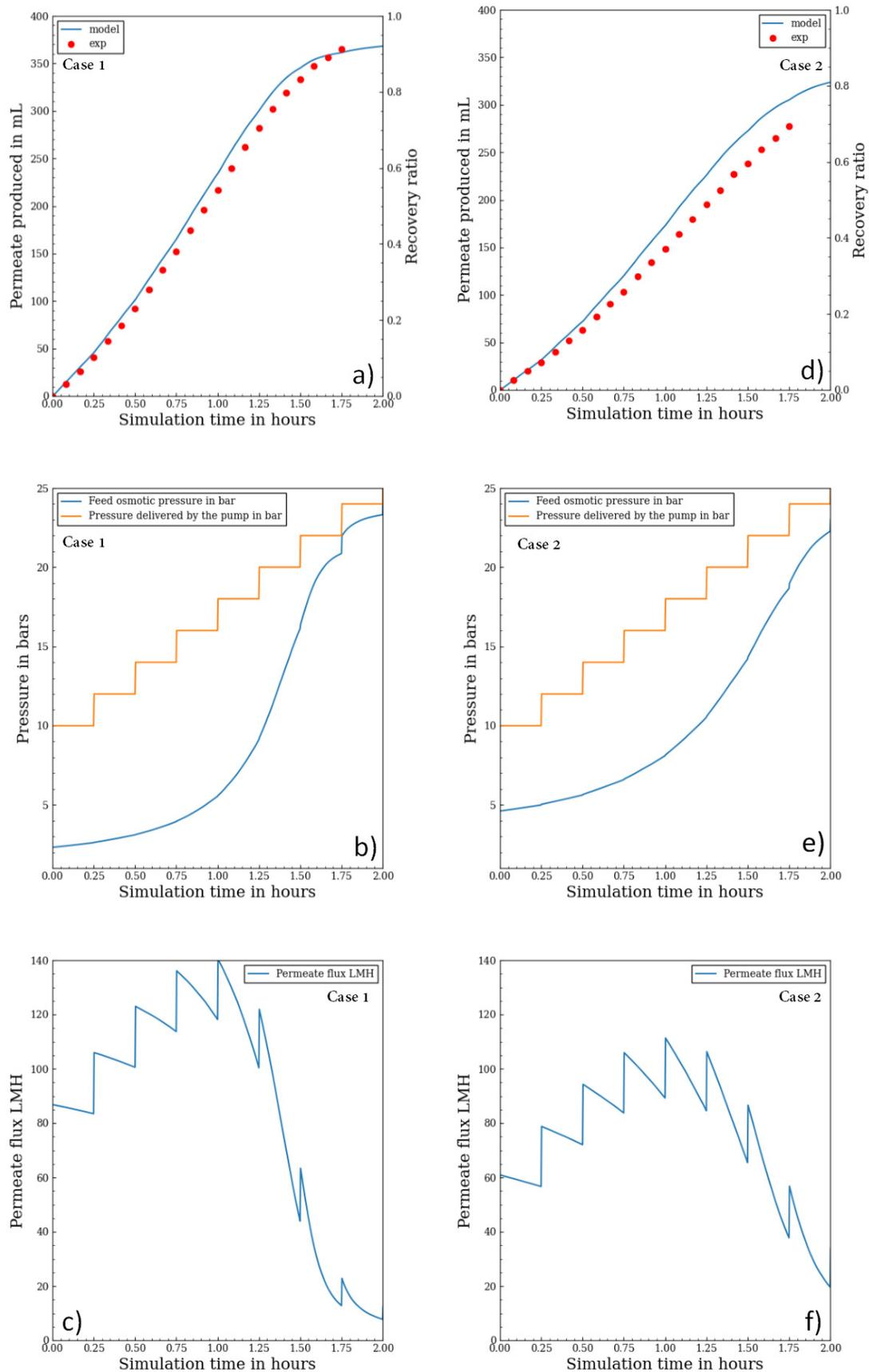
**Figure 6.** (a) and (d) batch RO permeate volume production against time for the model and experiment, (b) and (e) batch RO model simulation of osmotic pressure and pump pressure evolution, (c) and (f) batch RO model simulation of permeate flux.
