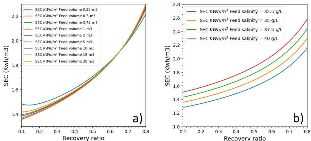
**Figure 9.** SEC batch RO process for seawater according to (a) feed volume and (b) feed salinity.
