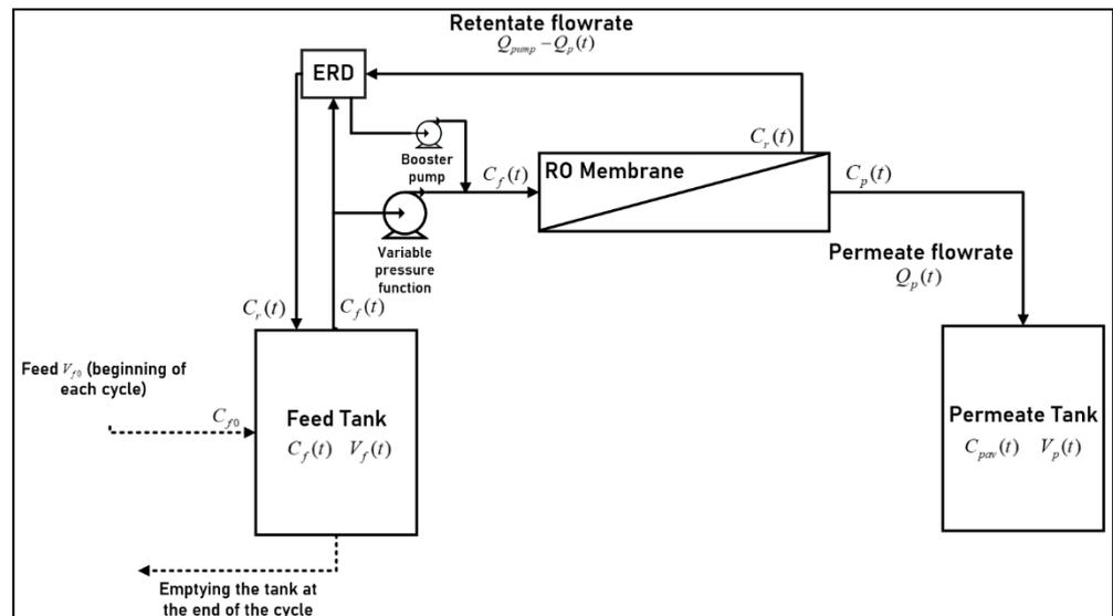
Figure 4. Schematic diagram of the batch RO process.
