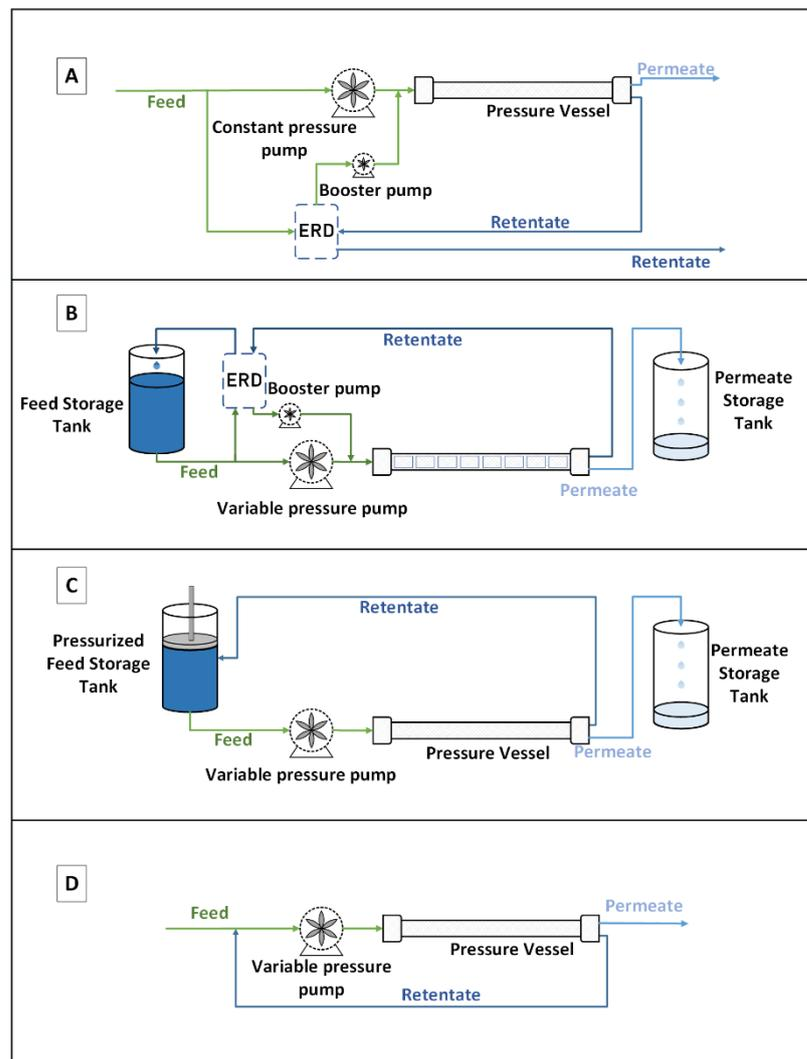
**Figure 1.** Schemes of four reverse osmosis (RO) desalination processes: Type A, one-stage continuous RO; Type B, batch RO with ERD and non-pressurized feed tank; Type C, batch RO with pressurized feed tank; Type D, semi-batch RO.
