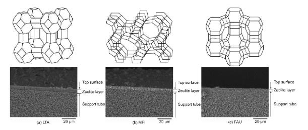
**Figure 3.** Schematic illustration of zeolite structures and SEM images of fractured sections of (**a**) LTA-, (**b**) MFI-, and (**c**) FAU-type zeolite membranes.
