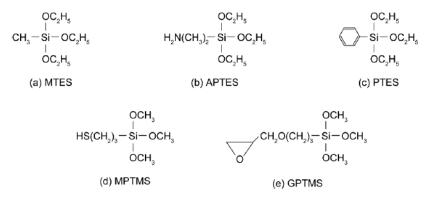
**Figure 1.** Silicon compounds using modification of FAU-type zeolite membrane in this study. (**a**) Methyltriethoxysilane (MTES), (**b**) 3-aminopropyltriethoxysilane (APTES), (**c**) phenyltriethoxysilane (PTES), (**d**) 3-mercaptopropyltrimethoxysilane (MPTMS), and (**e**) 3-glycidoxypropyltrimethoxysilane (GPTMS).
