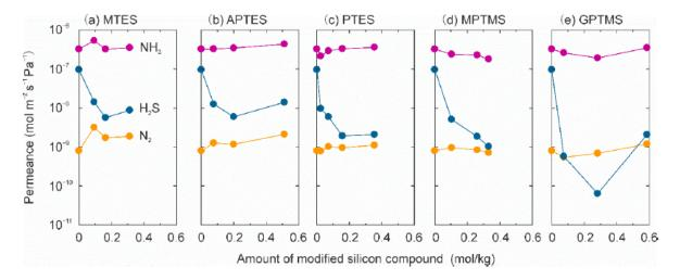
**Figure 8.** Effect of modification with silicon compounds on permeances of FAU-type zeolite membranes for ternary mixtures of NH<sub>3</sub>, H<sub>2</sub>S, and N<sub>2</sub> at 295 K. (a) MTES, (b) APTES, (c) PTES, (d) MPTMS, and (e) GPTMS.
