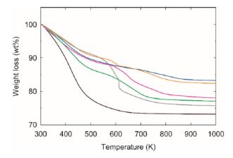
Figure 5. TG curves of non-modified (black), MTES-modified (blue), APTES-modified (red), PTES-modified (green), MPTMS-modified (orange), and GPTMS-modified (gray) FAU-type zeolite particles.
