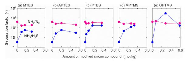
**Figure 9.** Influence of modification with silicon compounds on the separation factors of FAU-type zeolite membranes for ternary mixtures of NH<sub>3</sub>, H<sub>2</sub>S, and N<sub>2</sub> at 295 K. (a) MTES, (b) APTES, (c) PTES, (d) MPTMS, and (e) GPTMS.
