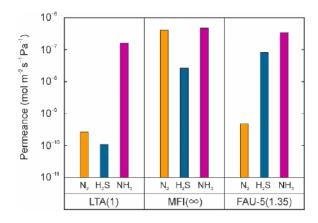
**Figure 6.** Effect of crystal structure of zeolite on gas permeation properties of membranes for ternary mixtures of NH<sub>3</sub>, H<sub>2</sub>S, and N<sub>2</sub> at 295 K.
