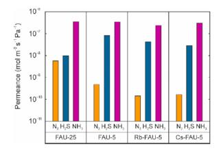
**Figure 7.** Effect of zeolite composition on gas permeation properties of FAU-type zeolite membranes for ternary mixtures of NH<sub>3</sub>, H<sub>2</sub>S, and N<sub>2</sub> at 295 K.
