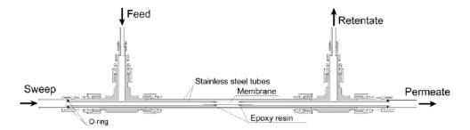
Figure 2. Schematic illustration of the permeation cell.
