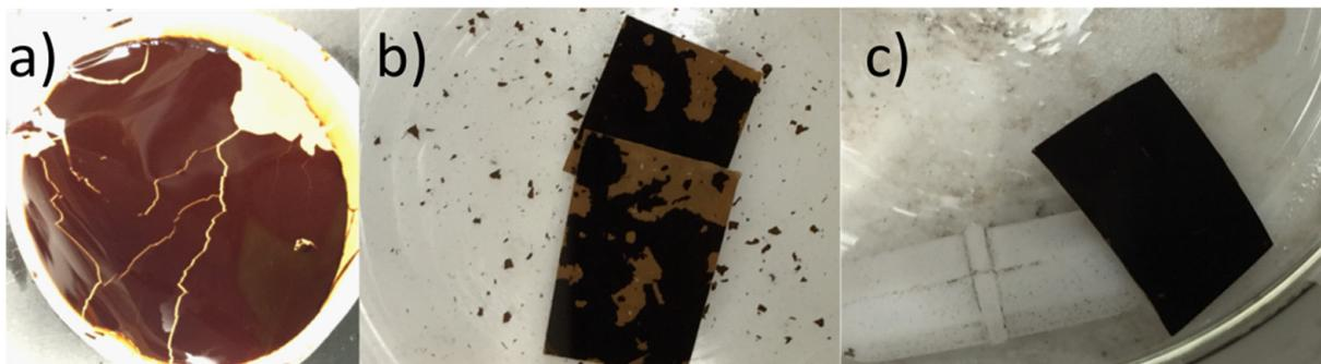
**Figure 3.** Membrane stability enhancement by  $\text{Zn}^{2+}$  crosslinking: (a) vacuum filtered GO membrane immersed in water for 30 min; (b,c) squares of membrane exposed to high speed mechanical stirring with no zinc treatment: squares in (b) have no  $\text{Zn}^{2+}$  treatment while the membrane in (c) was soaked in the  $\text{Zn}^{2+}$  solution for 24 h.
