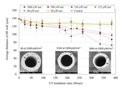
**Figure 1.** Average thickness of HFs' wall after UV irradiation in UP water with various irradiation powers. Insert: SEM images of HFs irradiated at 1000  $\mu$ W/cm<sup>2</sup> during 8 h, 216 h or 384 h (×350 magnification).
