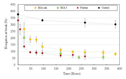
**Figure 9.** Elongation at break measured on UV irradiated HFs (1000  $\mu$ W/cm<sup>2</sup>). Pristine HFs (**red dots**), BSA<sub>ads</sub> HFs (**yellow squares**) and BSA<sub>f</sub> HFs (**green squares**). Control (**black dots**) = pristine HFs without UV irradiation.
