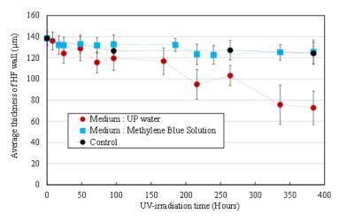
**Figure 4.** Average thickness of HFs' wall after UV irradiation at 1000  $\mu$ W/cm<sup>2</sup> in an MB solution (**blue squares**), in UP water (**red dots**). Control is non-irradiated HFs in am MB solution (**black dots**).
