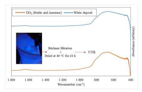
**Figure A1.** FTIR spectra of commercial TiO<sub>2</sub> used in the production of the membrane (**orange**) and of the dried white deposit observed in the soaking medium (**blue**).
