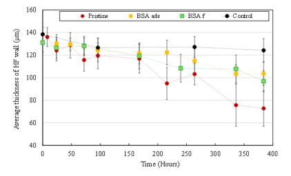
**Figure 8.** Average thickness of HFs' wall after UV irradiation at 1000  $\mu$ W/cm<sup>2</sup>. Pristine HFs (**red dots**), BSA pre-adsorbed HFs (**yellow squares**) and BSA pre-filtrated HFs (**green squares**). Control (**black dots**) = pristine HFs without UV irradiation.
