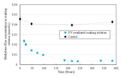
**Figure 6.** MB concentration in liquid samples collected from the soaking medium of irradiated HFs (**blue squares**) and non-irradiated control HFs (**black dots**).
