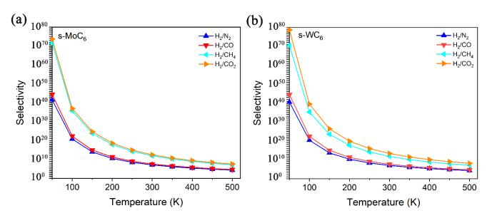
**Figure 5.** Selectivity versus temperature for  $H_2/N_2$ ,  $H_2/CO$ ,  $H_2/CH_4$ , and  $H_2/CO_2$  separation by (a) s-MoC<sub>6</sub>, (b) s-WC<sub>6</sub>.
