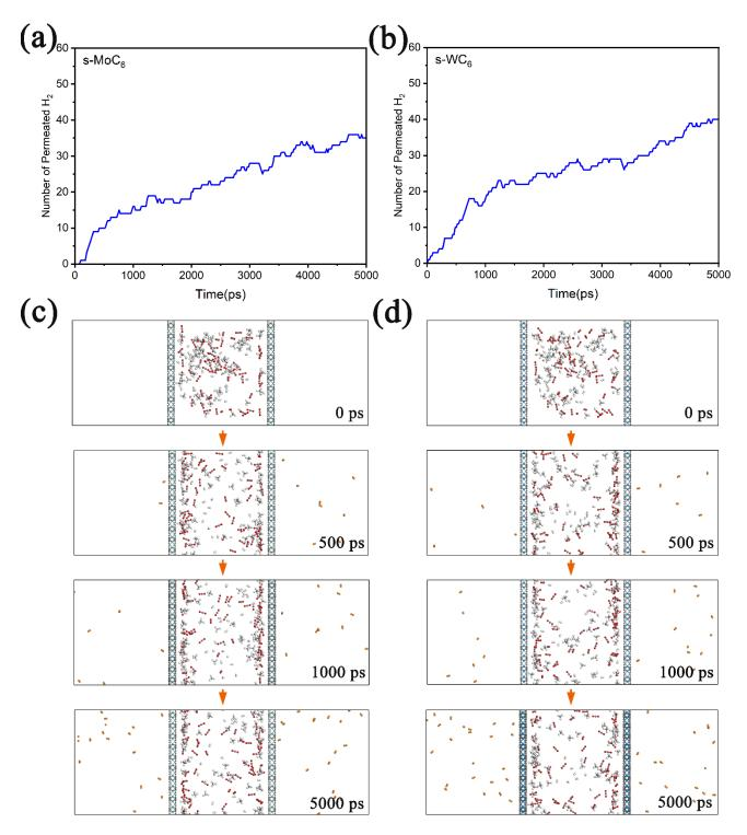
**Figure 6.** The number of permeated  $H_2$  molecules versus the simulation time for gas mixture in chamber composed of (**a**) s-MoC<sub>6</sub> membranes and (**b**) s-WC<sub>6</sub> membranes. Corresponding snapshots of the diffusion process (from 0 to 5000 ps) of gas mixture permeating through (**c**) s-MoC<sub>6</sub> membranes and (**d**) s-WC<sub>6</sub> membranes. The  $H_2$  molecules that diffuse outside are displayed by different color.
