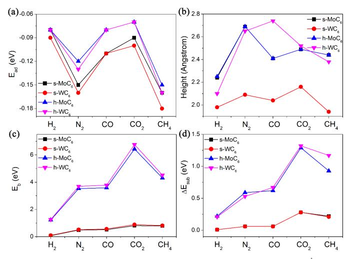
**Figure 2.** (a) The adsorption energies ( $E_{ad}$ , eV), (b) equilibrium adsorption heights (h, Å), (c) diffusion barriers for the studied gases (H<sub>2</sub>, N<sub>2</sub>, CO, CO<sub>2</sub>, and CH<sub>4</sub>) passing through the intrinsic pore ( $E_b$ , eV) of 2D TMC<sub>6</sub>, and (d) energy differences ( $\Delta E_{sub}$ , eV) of the TMC<sub>6</sub> membranes between free-standing state and TS without adsorbates.
