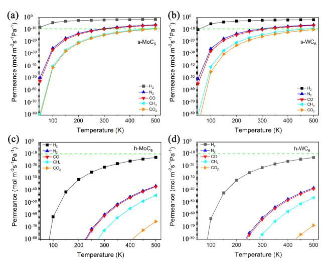
**Figure 4.** Permeance versus temperature for  $H_2$ ,  $N_2$ , CO, CO<sub>2</sub>, and CH<sub>4</sub> passing through the intrinsic pore of (**a**) s-MoC<sub>6</sub>, (**b**) s-WC<sub>6</sub>, (**c**) h-MoC<sub>6</sub>, and (**d**) h-WC<sub>6</sub>.
