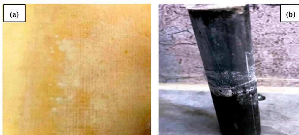
**Figure 12.** Accumulation of salts on the surface of the membrane and cathode electrodes after the end of the electro-kinetic process (EK-4 and membrane). (a) Membrane; (b) cathode electrode.
