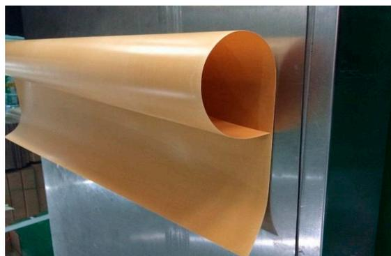
**Figure 2.** Cation exchange flat sheet membrane [17].
