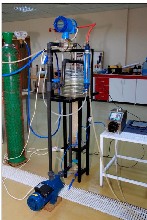
**Figure 5.** The developed membrane draft tube jet loop reactor.
