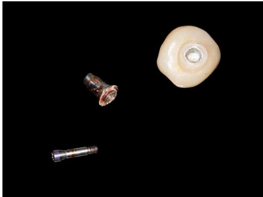
**Figure 2.** Fracture of a ti-base abutment after 3.75 years of service.
