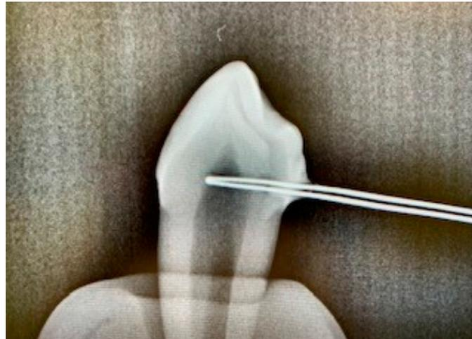
**Figure 3.** X-ray control image to assess the correct position of the thermocouple.
