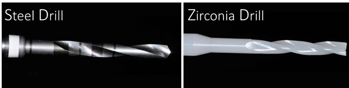
**Figure 1.** Steel cylindrical 2 mm diameter drill and zirconia cylindrical 2 mm diameter drill used for the investigation.
