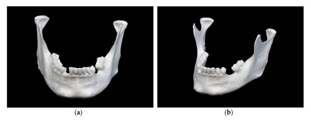
**Figure 3.** Mandibular model printed in fused filament fabrication (FFF) technology: (a) front view; (b) side view.
