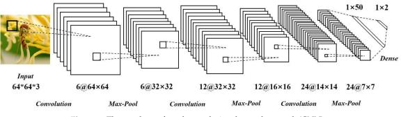
Figure 4. The topology of used convolutional neural network (CNN).
