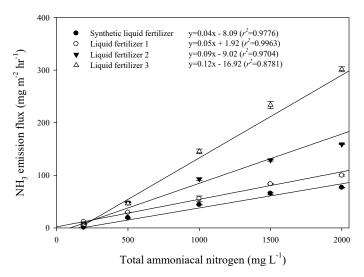
**Figure 2.** Changes in ammonia emission flux by liquid fertilizer type using a dynamic chamber-capture system at  $20^{\circ}$ C and pH 8 condition. Error bar means standard deviation (SD, n = 3).
