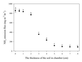
**Figure 3.** Changes in ammonia emission flux with different soil media thickness using dynamic chamber-capture system at 20 °C and pH 8 condition. Means with different letters are significantly different (Tukey's test, p < 0.05). Error bar means standard deviation (SD, n = 3).
