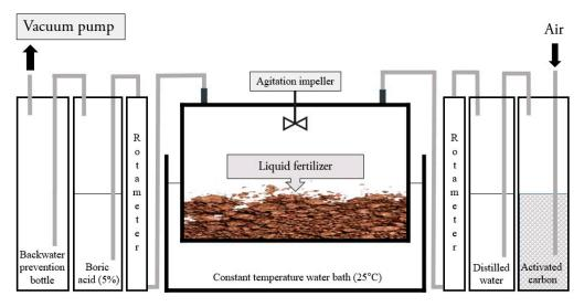
Figure 1. Schematic of dynamic chamber-capture system (DCS) with a constant temperature water bath.
