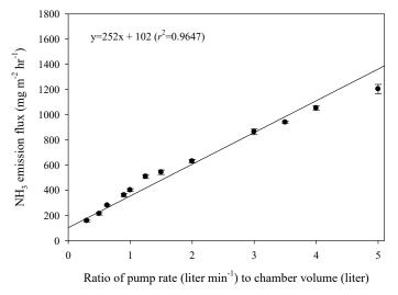
**Figure 4.** Changes in ammonia emission flux with different ventilation rate (min<sup>-1</sup>) using dynamic chamber-capture system at 20 °C condition. Error bar means standard deviation (SD, n = 3).
