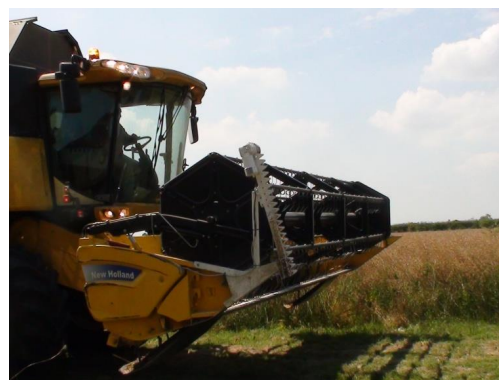
Figure 2. Modified wheat header for canola harvesting (photo by Authors).
