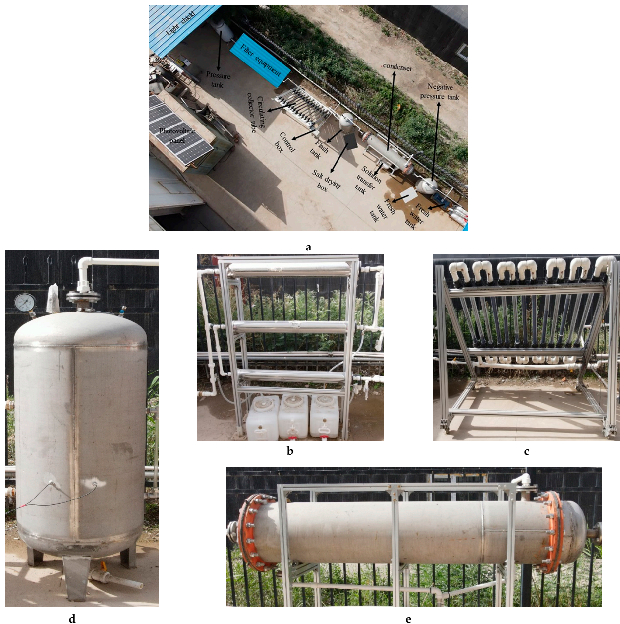
Figure 6. Installation environment of farmland saline alkaline water separation and desalination device: (a) general drawing of farmland saline alkaline water separation and desalination unit; (b) NF-RO device; (c) circulating solar collector tube; (d) flash tank; (e) shell-and-tube circulating condenser.
