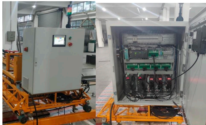
Figure 13. (a) Physical relation diagram of the control system of the tray laying machine. (b) Control electrical cabinet of tray laying machine.
