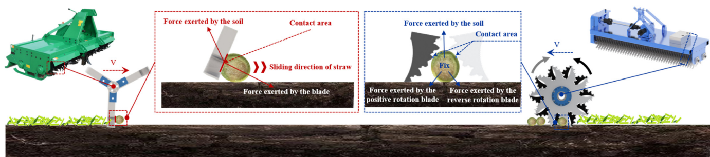
Figure 6. Comparison of the operating principle between traditional straw returning machine and bionic straw returning machine. The straw slips during the operation of traditional straw returning machine, and the contact area between the blade and the straw is large. During the operation of the bionic straw returning machine, the straw is fixed and the contact area between the blade and the straw is smaller.
