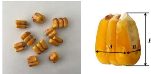
**Figure 5.** Adhering kernels and their characteristic dimensions.
