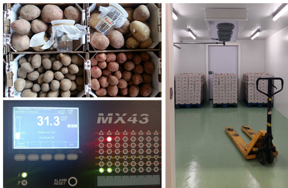
Figure 2. Commercial trial. Pallet preparation using inoculated potatoes with eggs and larvae, pupae, and adults in cylindrical vases, and one box of healthy and another of infested potatoes classified by the farmer. Photos: M.G. Lobo.
