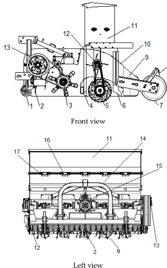
**Figure 1.** Structure of strip fertilization planter for straw back throwing and inter-row laying. 1—depth limiting wheel; 2—protection curtain; 3—crushing spindle; 4—fertilization port; 5—rotary tillage spindle; 6—seed port; 7—suppression wheel; 8—scraper board; 9—diversion device; 10—cover plate; 11—seed fertilizer box; 12—fan shaft; 13—transmission mechanism; 14—frame; 15—reducer; 16—fertilizer fluted roller; 17—seed fluted roller.
