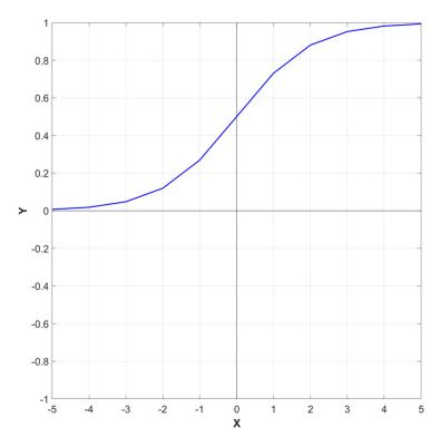
Figure 7. Graphic illustration of logistic sigmoid activation function.
