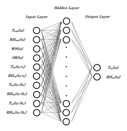
Figure 8. Scheme of the neural network structure.
