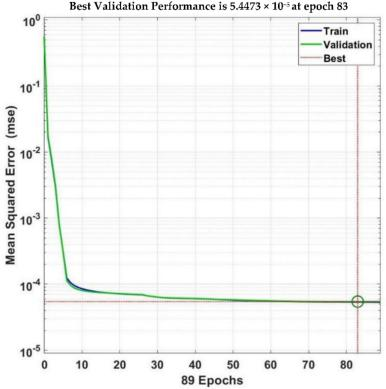
Figure 10. Convergence of mean square error with epochs throughout training and validation process.
