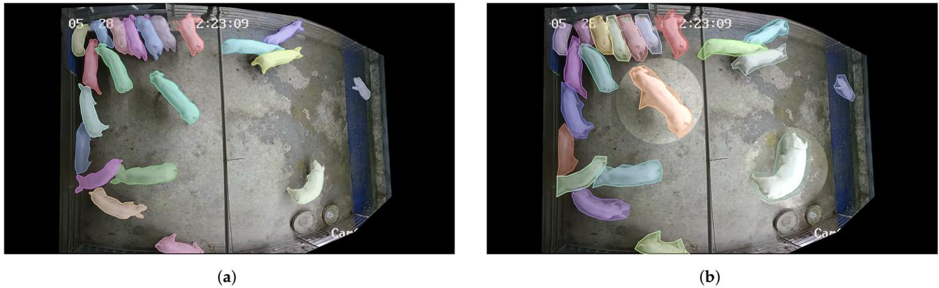
**Figure 3.** Comparison of semi-auto and manual annotation methods. (a) Semi-auto annotation (96 points, 5s per instance). (b) Manual annotation (17 points, 35s per instance).
