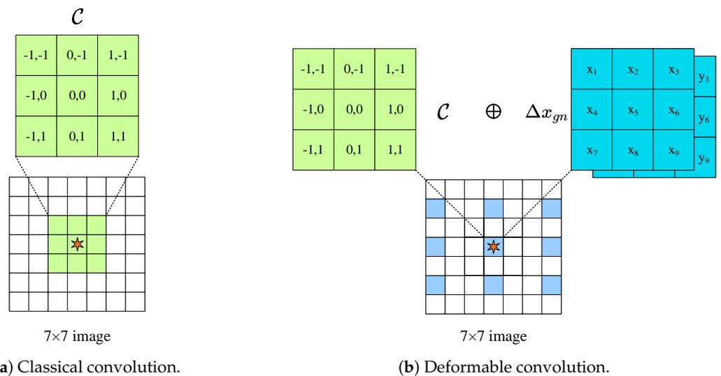
**Figure 7.** Examples displayed under  $3 \times 3$  kernel within  $7 \times 7$  image. The pentagram of image represents the center of convolution. The green and blue squares in these two  $7 \times 7$  images represent the receptive field range of current convolution.
