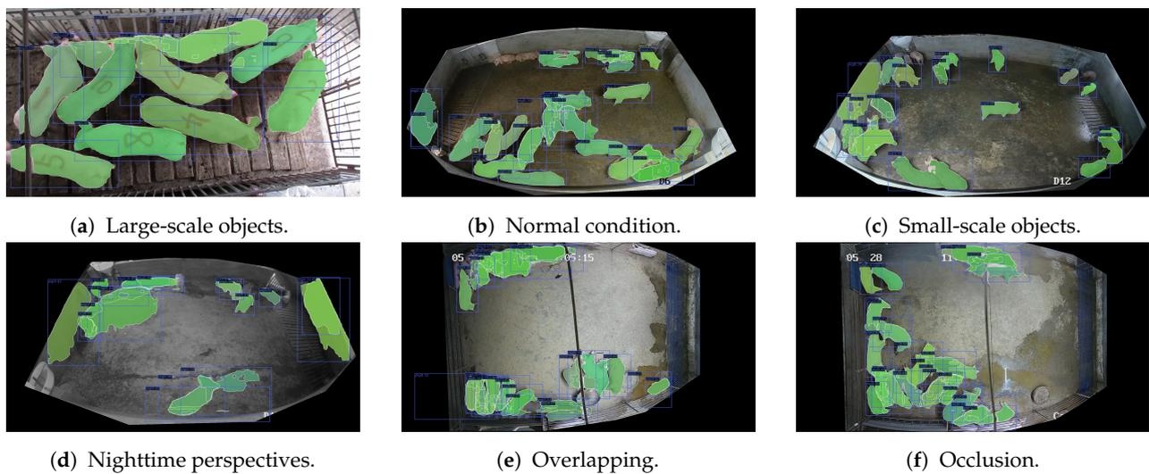
**Figure 8.** Visualization results of test set including different situations based on Mask R-CNN. The numbers on pigs of subfigure (a) represent the identifiers of pigs.
