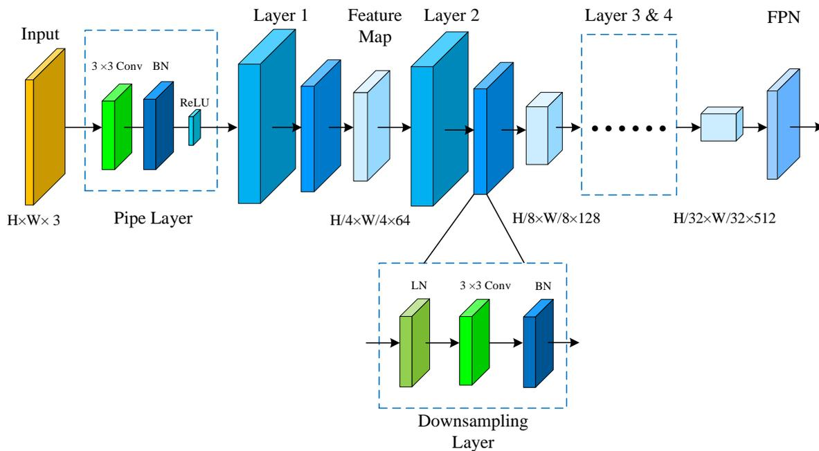
**Figure 5.** The overall structure of the ICNet, where BN and LN stand for Batch Normalization and Layer Normalization, respectively.
