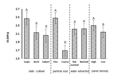
**Figure 7.** Effect of date palm cultivar, particle size, hot water extraction and panel density on internal bond (IB) property. (Means with same letter do not significantly different at L.S.D.<sub>0.05</sub>).
