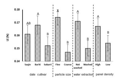
**Figure 8.** Effect of date palm cultivar, particle size, hot water extraction and panel density on linear expansion (LE) property. (Means with same letter do not significantly different at L.S.D.<sub>0.05</sub>).
