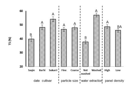
**Figure 9.** Effect of date palm cultivar, particle size, hot water extraction and panel density on thickness swelling (24-h TS) property. (Means followed by with same letter do not significantly different at L.S.D.<sub>0.05</sub>).
