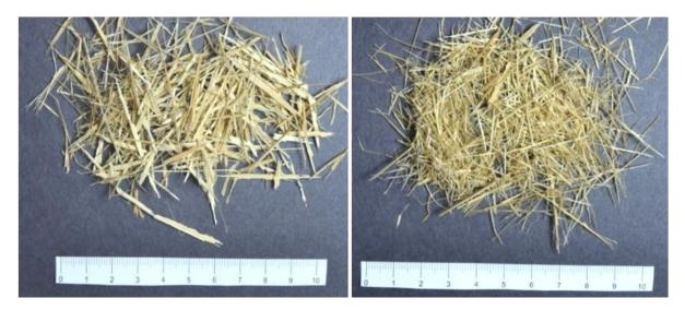
Figure 3. Coarse and fine date palm frond particles used in this study.
