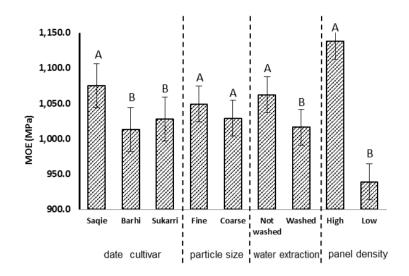
**Figure 6.** Effect of date palm cultivar, particle size, hot water extraction and panel density on Modulus of Elasticity (MOE) property. (Means with same letter do not significantly different at L.S.D.<sub>0.05</sub>).
