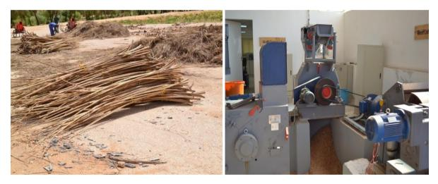
Figure 1. Date palm fronds without leaflets and the ring flaker machine (BX-466).
