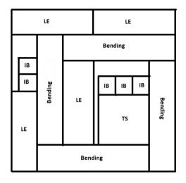
**Figure 2.** Cutting diagram for mechanical and physical samples taken from the manufactured panels (48 × 48 cm). Bending samples =  $32 \times 7.5$  cm, internal bond (IB) =  $5 \times 5$  cm, linear expansion (LE) =  $24 \times 7.5$  cm, thickness swelling and water absorption (TS) =  $15 \times 15$  cm.
