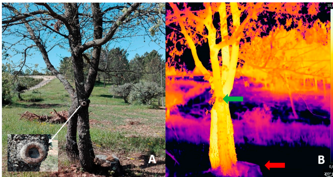
Figure 8. Photo (A) and thermogram (B) of the Quercus pyrenaica Willd tree. The white arrow shows an enlarged image of the CODIT development wall; the green arrow shows the same wall of CODIT on the thermogram; the red arrow indicates a stump. CODIT: compartmentalization of decay in trees.
