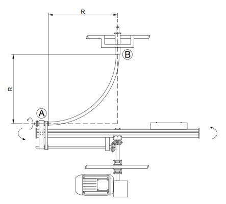
**Figure 3.** The test rig setup with cable mounted. The cable is fixed at the top, and the rotating end is controlled via a mechanical drive visible at the bottom of the picture (A and B are end points, see the text for clarification).
