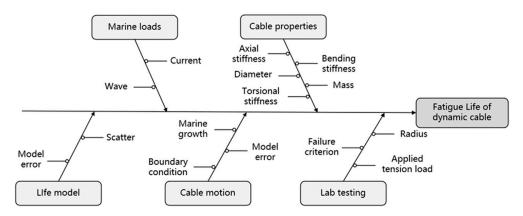
**Figure 6.** Ishikawa diagram [32] for the given uncertainty sources for the VMEA application of flexible power cable reliability and fatigue assessment process design.
