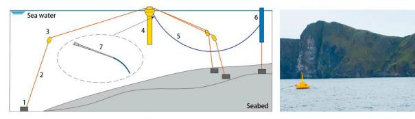
**Figure 1.** (**Left**) Illustration of the WaveEL 3.0 installation in Runde: (1) gravity anchor, (2) segment of a mooring line, (3) floater, (4) WEC, (5) cable, (6) hub, (7) bending restrictor, and (**right**) the full-scale WaveEL 3.0 system (photograph taken by the fourth author).
