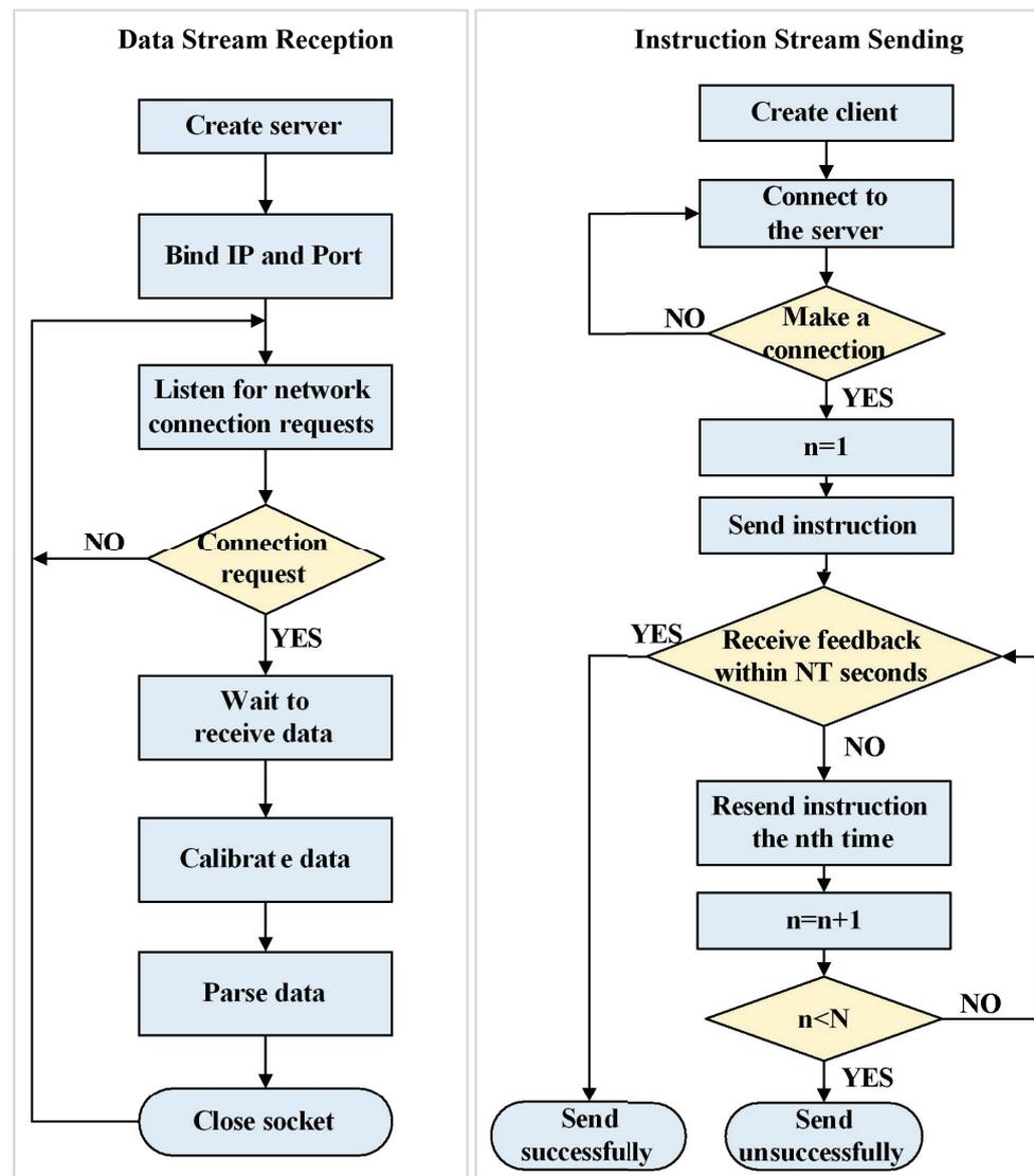
Figure 3. The flow chart of bidirectional socket network communication.
