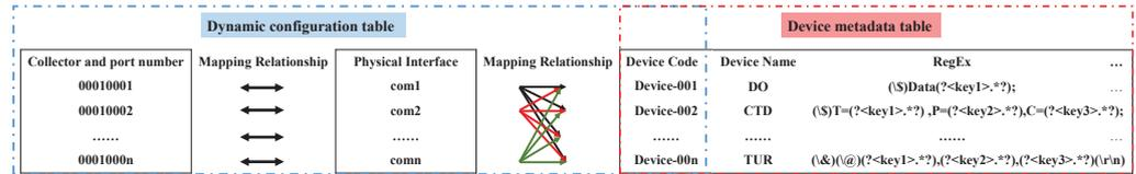
Figure 6. The mapping diagram of dynamic device management.
