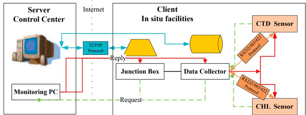
Figure 2. The C/S architecture and remote communication of SON-MS.
