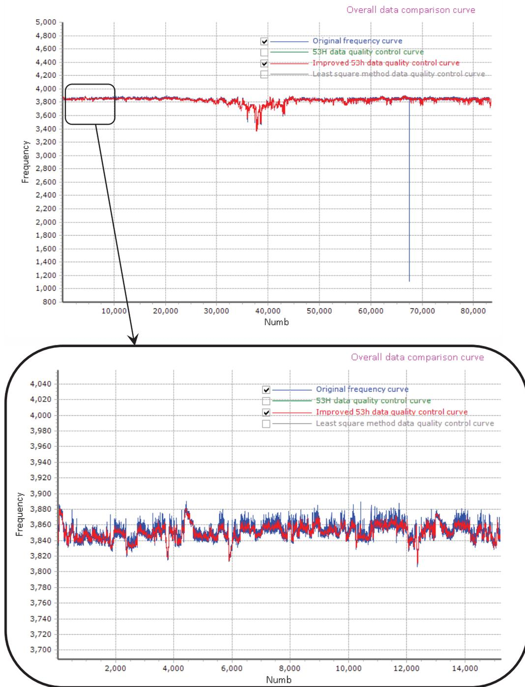
Figure 13. The filtering results of the improved 53H algorithm.
