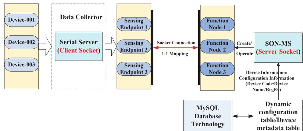
**Figure 5.** The mechanism diagram of an underwater device, data collector and SON-MS.
