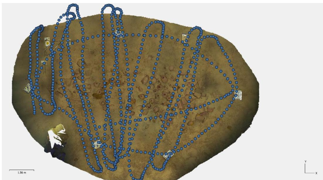
**Figure 9.** Image of the flypath covered by 3D dive. The blue circles indicate the position of the camera when the photo was taken, creating a flypath of how the diver recorded the site. © University of Malta.
