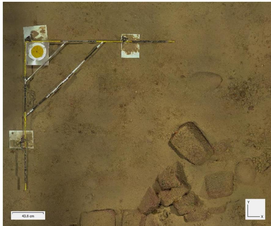
**Figure 7.** Image of reference square set up to capture the inclination of the seabed. © University of Malta.
