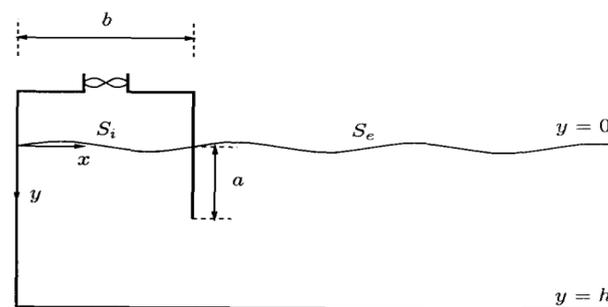
**Figure 6.** Oscillating water column ([24] 1995).
