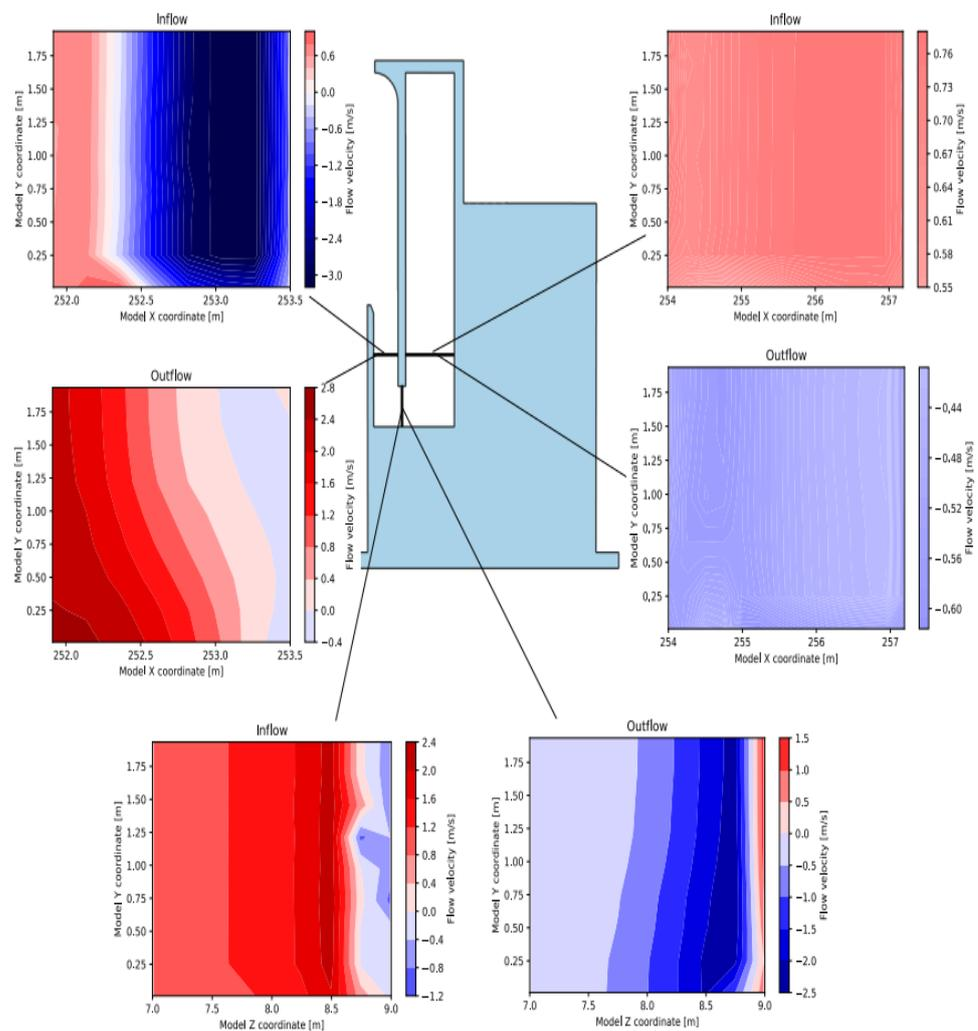
Figure 22. The flow velocity pattern within the cylinder ([97] 2021).
