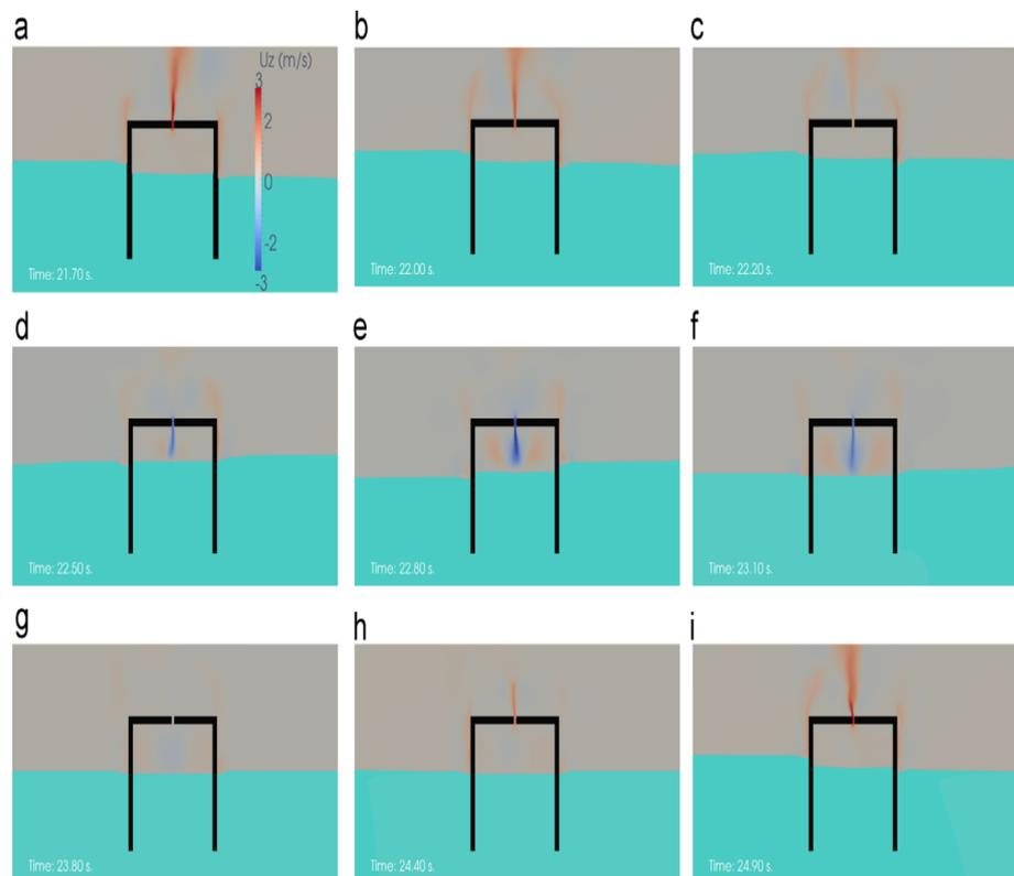
Figure 20. The vertical air velocity within the chamber throughout a pressurization–depressurization cycle (a)  $t = 21.70$  s; (b)  $t = 22.00$  s; (c)  $t = 22.20$  s; (d)  $t = 22.50$  s; (e)  $t = 22.80$  s; (f)  $t = 23.10$  s; (g)  $t = 23.80$  s; and (h)  $t = 24.40$  s; and (i)  $t = 24.90$  s ([94] 2015).
