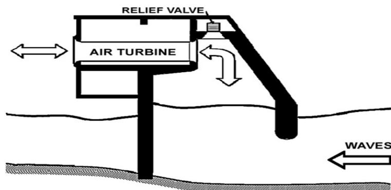
**Figure 5.** A view showing the cross-section of a bottom-standing OWC (Pico plant).
