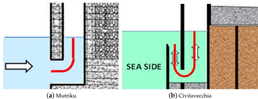
Figure 15. Cross-section of the Mutriku conventional OWC and the U-shaped OWC of Civitavecchia breakwater ([90] 2022).
