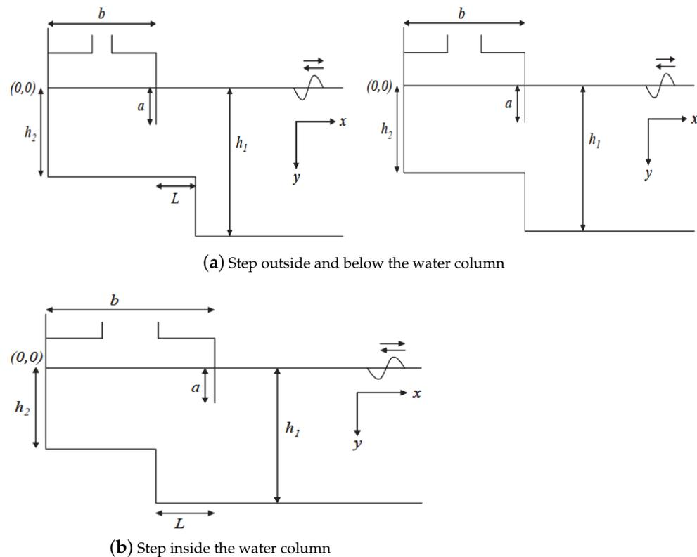
**Figure 7.** Single oscillating water column ([62] 2013).
