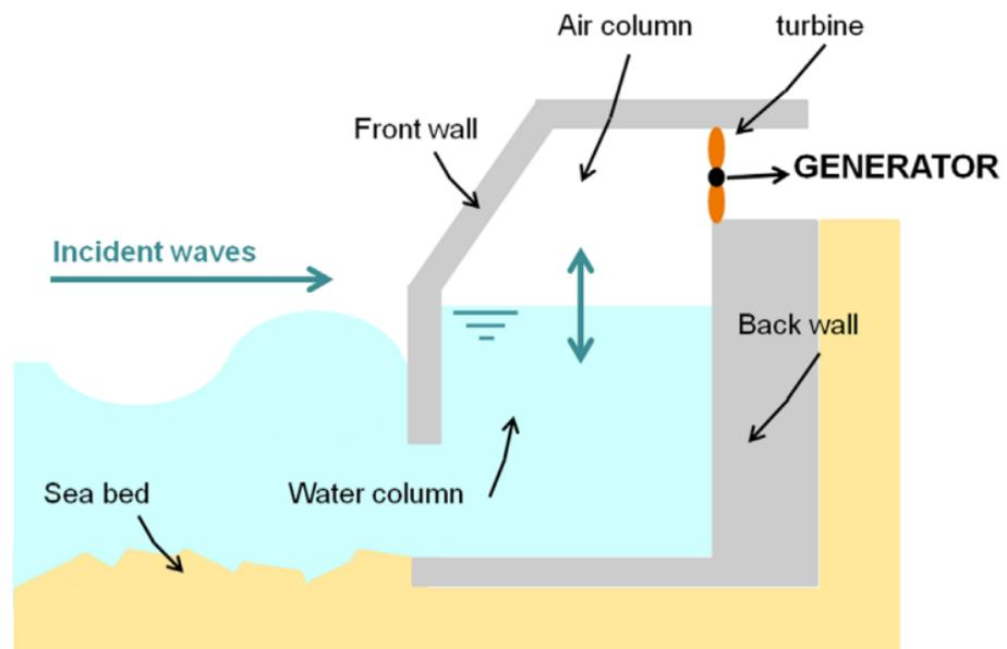
Figure 19. The oscillating water column scheme ([94] 2015).
