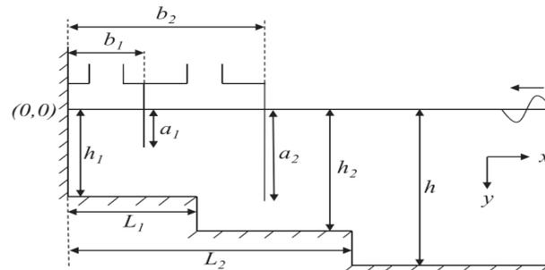
Figure 9. Dual chamber OWC ([75] 2015).
