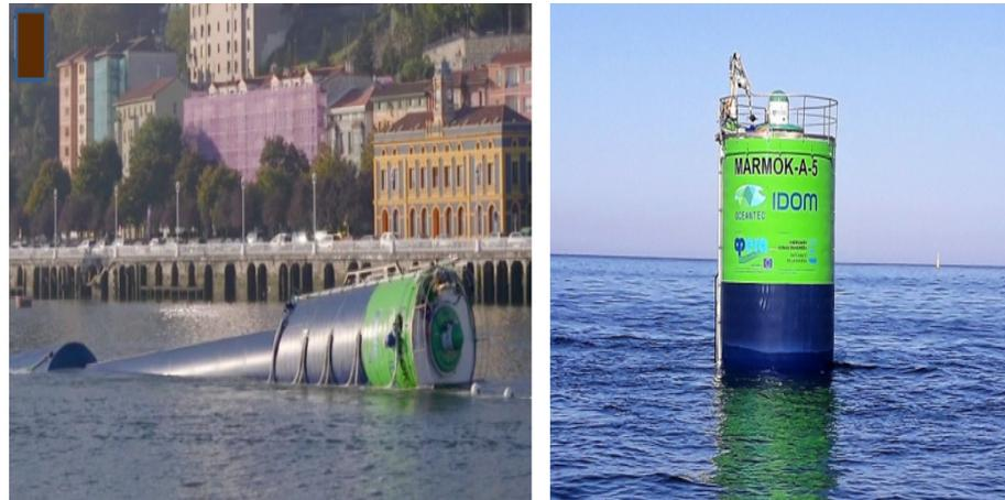
**Figure 17.** MARMOK-A-5 spar-buoy OWC Spain [90]).
