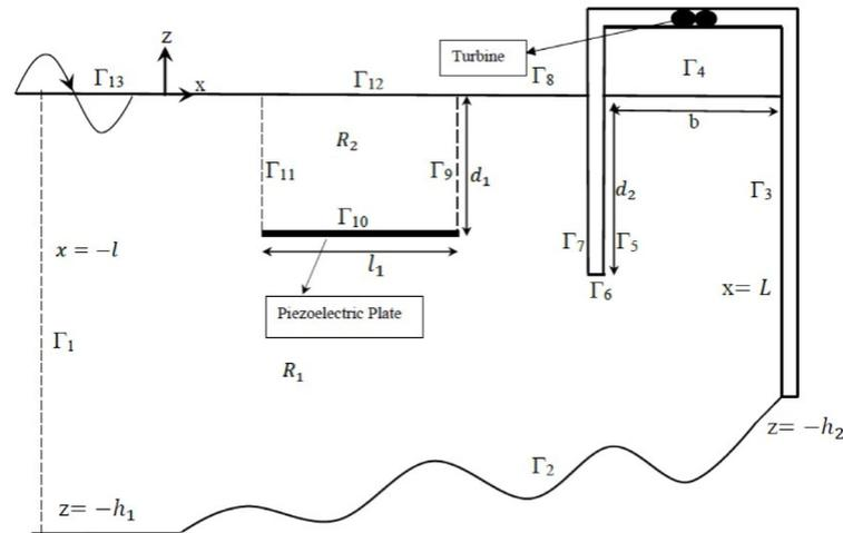
Figure 8. Piezoelectric plate and the OWC device placed over an undulated seabed ([68] 2023).
