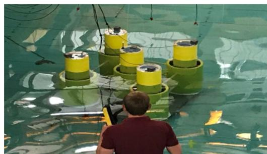
**(c)** Experimental Testing of Array in the Wave Tank
