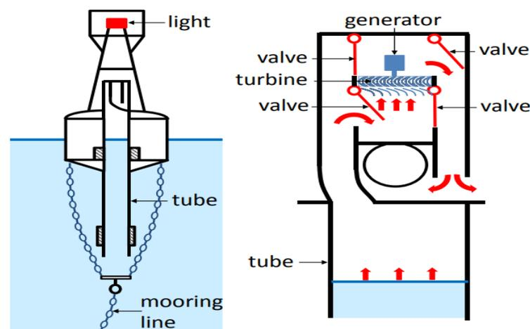
**Figure 1.** Layout of Masuda's navigation buoy ([37] 2006). The airflow via the rectifying and turbine valves is shown in detail on the right.
