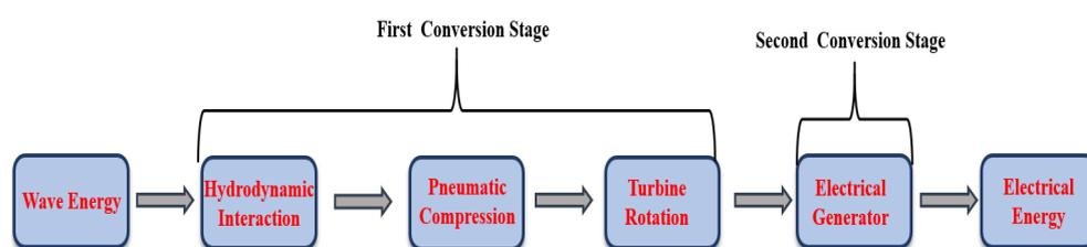
**Figure 4.** Working principle of OWC ([38] 2019).
