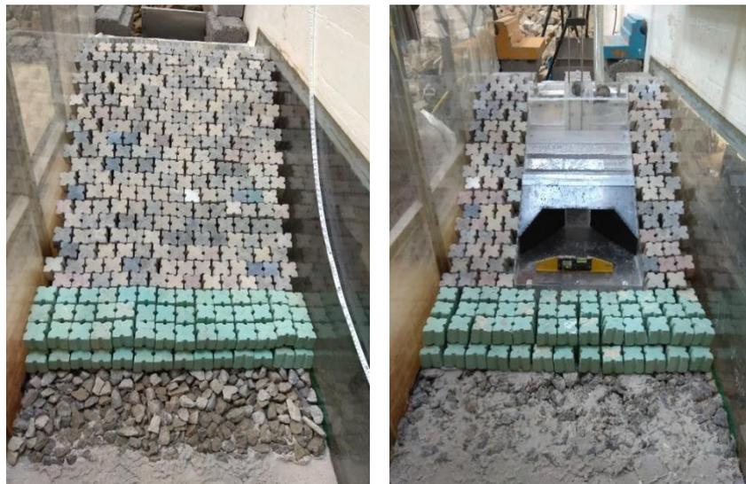
**Figure 8.** Physical model without (left) and with (right) the hybrid WEC module (geometry B) integrated in the breakwater and before the experimental tests.
