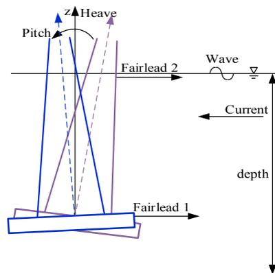
**Figure 8.** Schematic view of the pitch and heave motion directions, the loading environments and the fairlead positions.
