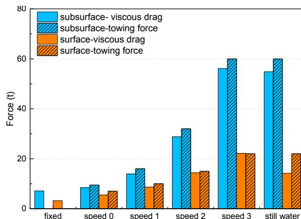
**Figure 7.** Comparison between the surface towing and the submerged towing under different towing speeds in terms of the viscous drag force and the towing force.
