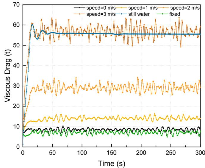
**Figure 6.** Comparison between the time history curves of the viscous drag force under different towing speeds for submerged towing (submerged depth: 40 m).
