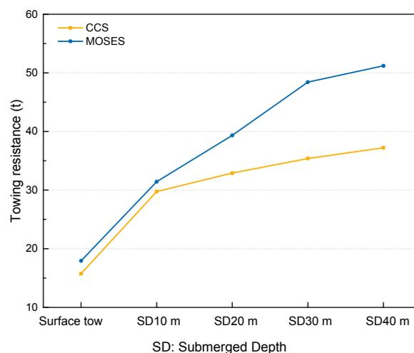
Figure 3. Towing resistances by two method (MOSES and CCS code) under surface tow and submerged tow.
