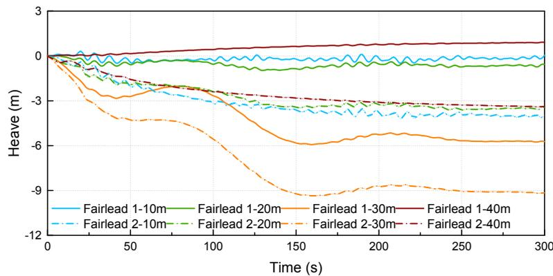
Figure 13. Heave motion versus fairlead positions under different submerged depths.
