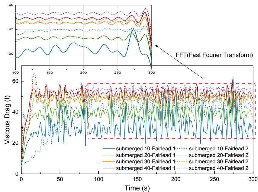
**Figure 10.** Comparison between the time history curves of the viscous drag force under different submerged depths in terms of the fairlead position (towing speed: 3 m/s).
