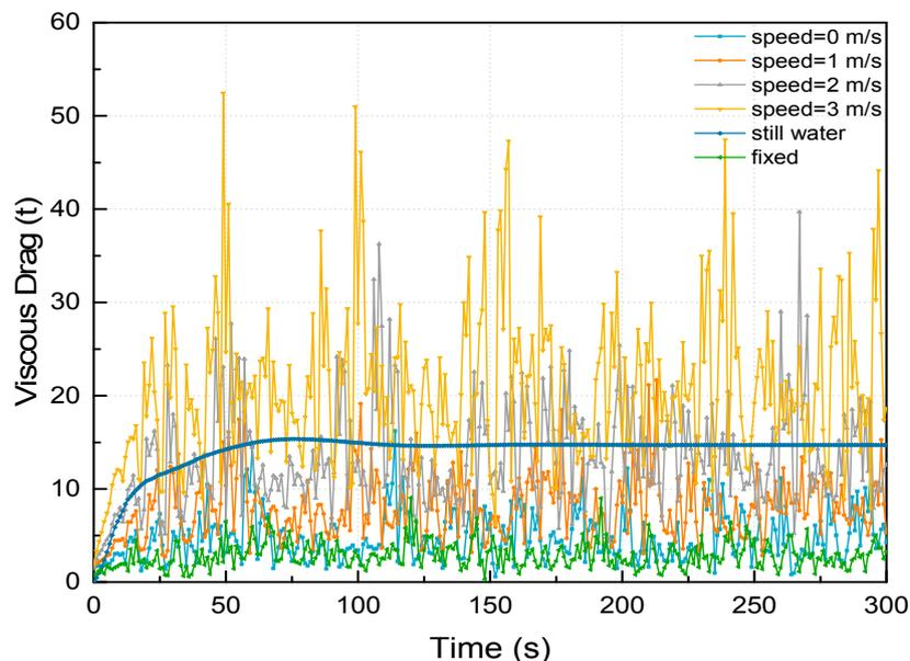
**Figure 5.** Comparison between the time history curves of the viscous drag force under different towing speeds for surface towing.
