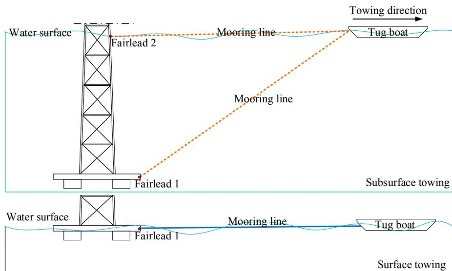
**Figure 2.** Surface towing and submerged towing methods.
