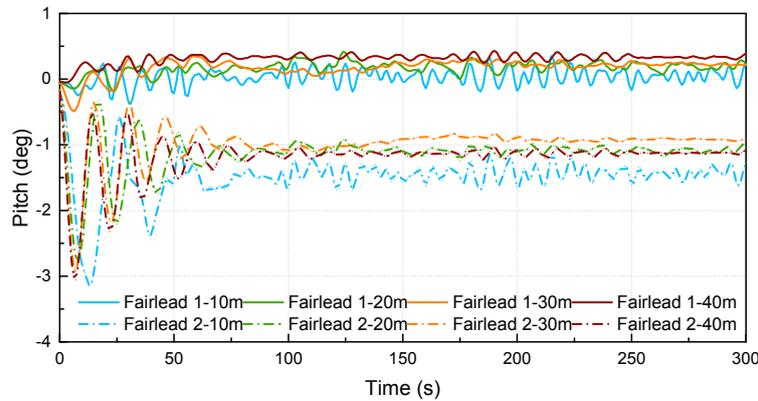
Figure 12. Pitch motion versus fairlead positions under different submerged depths.
