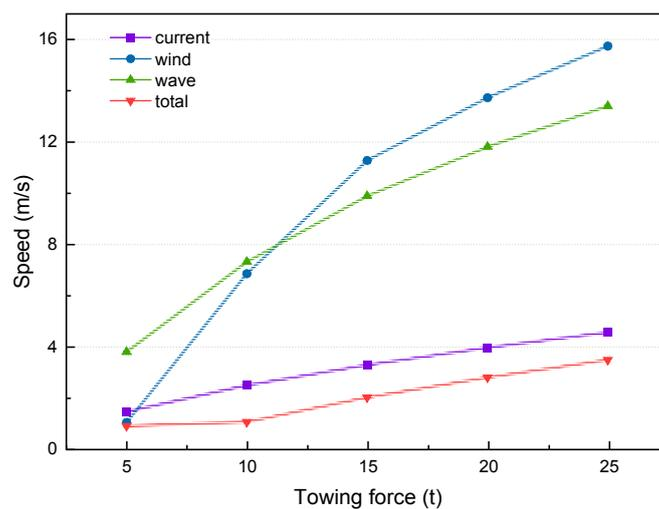
Figure 4. Comparison between the towing speed under different sea loads varying with the towing force by MOSES.
