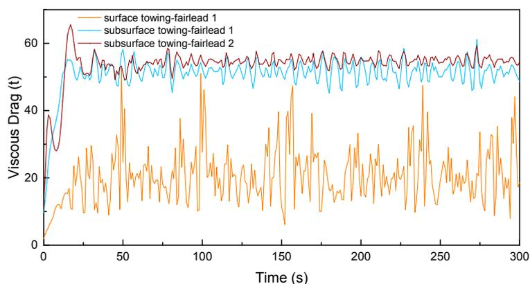
**Figure 9.** Comparison between the time history curves of the viscous drag force for surface towing and subsurface towing in terms of the fairlead position (towing speed: 3 m/s).
