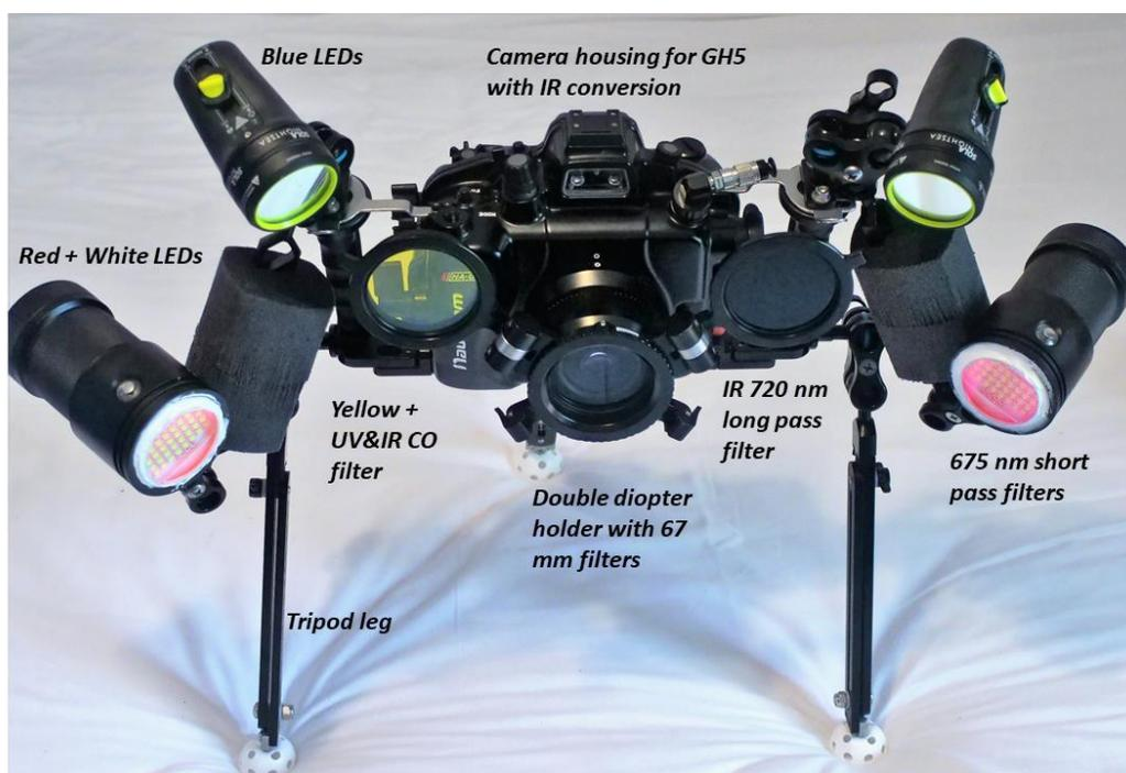
**Figure 1.** The imaging system used in this work showing the location of filters used. For all Chl imaging the white LEDs were used for excitation. For all GFP imaging, the blue LEDs were used. Each combination of lighting and filters required setting separate white balances before beginning.
