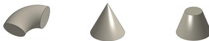
Figure 9. Basic type parts: elbow, cone, and truncated cone.
