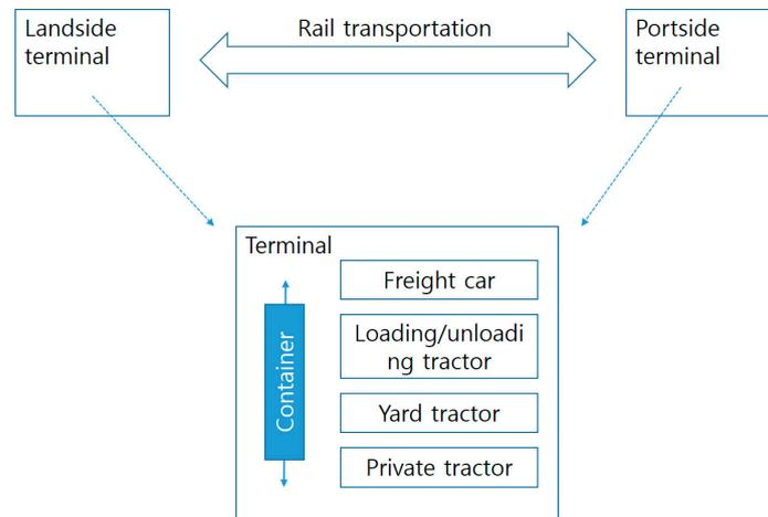
**Figure 1.** Conceptual diagram of the automated container transport system (ACTS).
