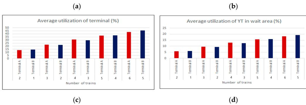
**Figure 18.** Simulation results for number of one-directional routes and avoidances by trains, as well as the travel times between terminals A and B, with a train operating time of 18 h: (a) number of containers on the train; (b) average waiting time of the train; (c) average utilization of the terminal; (d) average utilization of a yard tractor in the waiting area.
