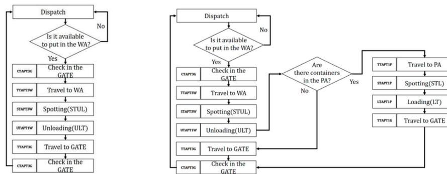
scenario 1: PT1 (yard chassis)- loading scenario 2: PT1 (yard chassis)- loading and unloading
