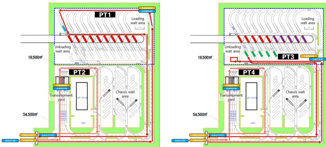
Figure 9. Operation logic for private tractor (left: loading; right: unloading).
