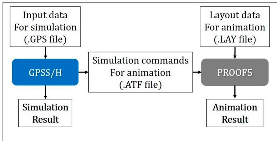
**Figure 5.** Method of integrating general-purpose simulation system/H (GPSS/H) simulation with PROOF5 animation.
