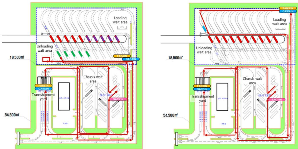
Figure 8. Operation logic for yard tractor (left: unloading; right: loading).
