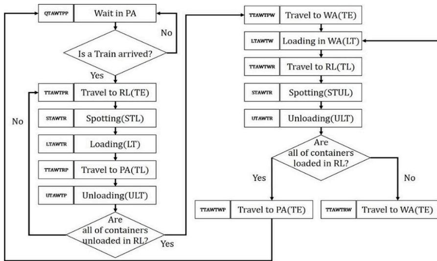
Figure 11. Simulation algorithm for loading/unloading tractor.
