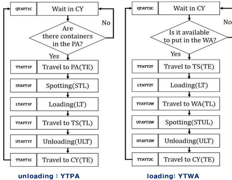
Figure 12. Simulation algorithm for yard tractor. YTPA and YTWA represent the yard tractors at the unloading and loading waiting areas, respectively.
