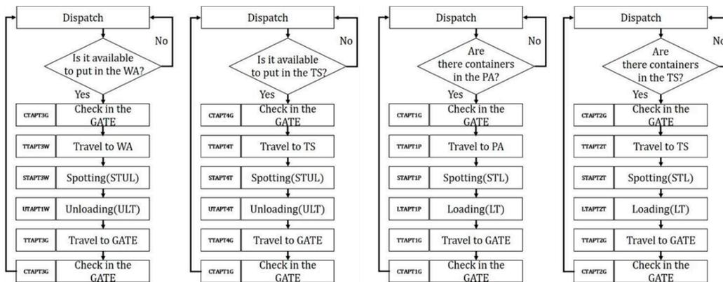
Figure 13. Simulation algorithm for private tractor (PT) (scenario 1 for yard chassis).
