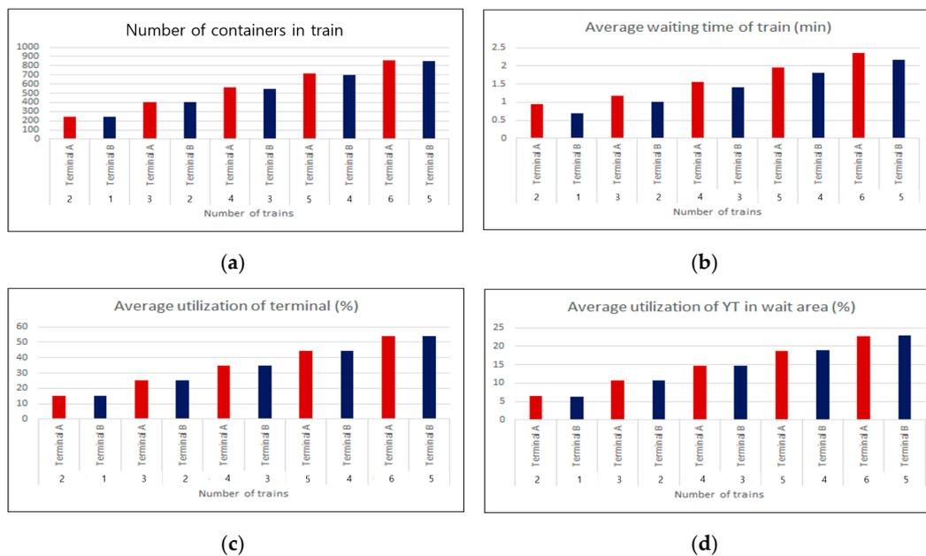
**Figure 19.** Simulation results for number of two-directional routes with trains, as well as the travel times between terminals A and B, with a train operating time of 18 h: (a) number of containers on the train; (b) average waiting time of the train; (c) average utilization of the terminal; (d) average utilization of a yard tractor in the waiting area.
