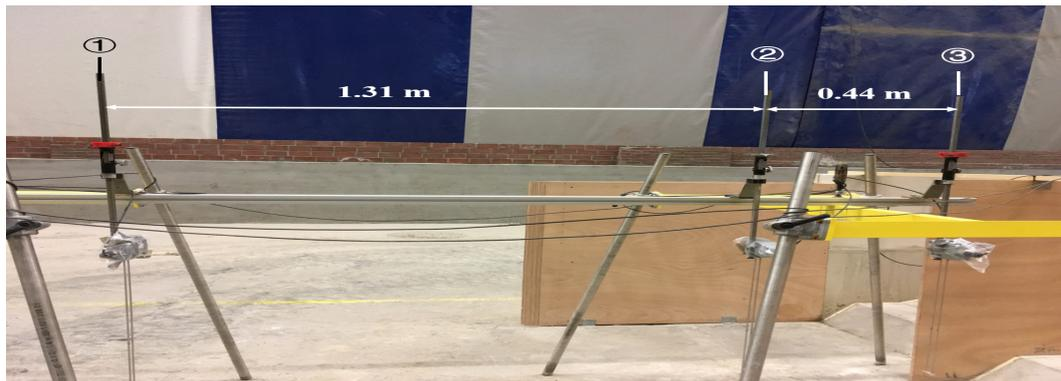
**Figure 4.** Experimental instruments for measurement with (a) wave gauges in front of models (side view) and (b) overtopping chute and overtopping tank with wave gauge (top view).
