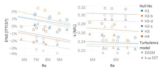
**Figure 10.** Comparison error of all test cases for the speed variations, (a) using the ITTC-57 line and (b) using the NFL.
