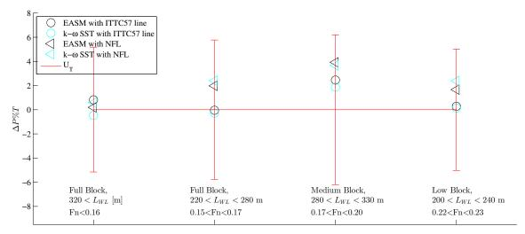
**Figure 17.** Relative change of the accuracy of the predictions,  $\Delta P\%T = 0$ , made with the CFD based form factors compared to the predictions with the standard ITTC-78 method, based on 18 test cases and 78 trials.
