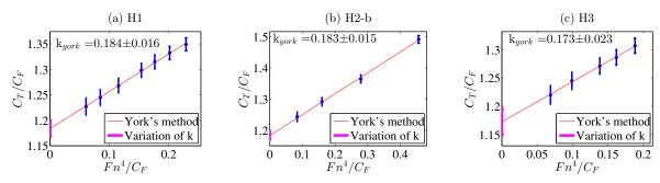
Figure 12. Prohaska plot of test cases in ballast loading condition: (a) H1, (b) H2-b, (c) H3.
