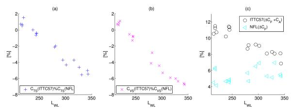
**Figure 18.** Difference between the (a)  $C_{TS}$ , (b)  $C_{VS}$  (including  $\Delta C_F + C_A$ ), and (c)  $\Delta C_F + C_A$  predictions using the CFD based form factors with the EASM turbulence model and different friction lines.
