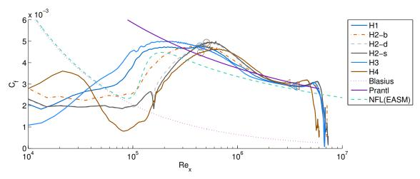
Figure 8. Local skin friction resistance coefficients for all hulls versus Reynolds number.
