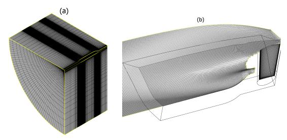
Figure 1. (a) Grid distribution of the coarsest grid, (b) grid refinement at the stern and the rudder as overlapping grids.
