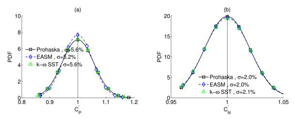
**Figure 14.** The probability density functions (PDFs) of the normalized correlation factors for the standard ITTC-78 method and using CFD-based form factors with two different turbulence models. (a)  $C_P'$  and (b)  $C_N'$ .
