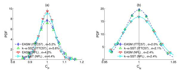
**Figure 15.** The probability density functions (PDFs) of the normalized correlation factors using the CFD based form factors with the ITTC-57 and the numerical friction lines. (a)  $C_P'$  and (b)  $C_N'$ .
