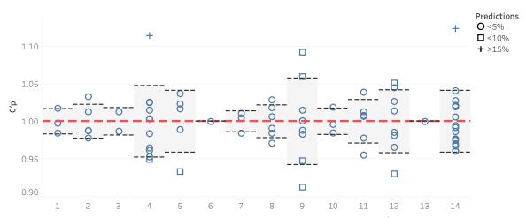
**Figure 16.** Illustration of the speed trial spread between sister ships for 14 ship series.  $C_P'$  values normalized to the mean of each series. Dashed black lines indicates the standard deviation.
