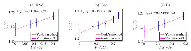
Figure 13. Prohaska plot of test cases in design and scantling loading conditions: (a) H2-d, (b) H2-d, (c) H4.
