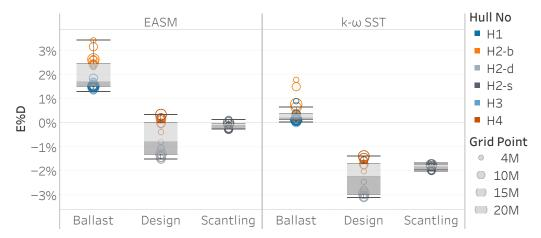
**Figure 11.** Comparison error of form factors for different loading conditions for the EASM and the  $k - \omega$  SST turbulence models.
