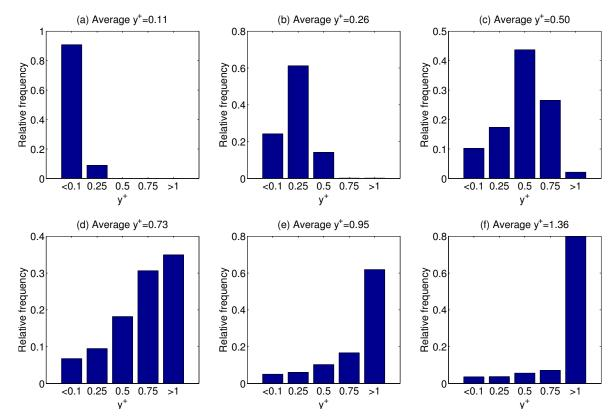
**Figure 4.** The histogram of the acquired  $y^+$  values for the H3 hull for the average (**a**)  $y^+ = 0.11$ , (**b**)  $y^+ = 0.26$ , (**c**)  $y^+ = 0.50$ , (**d**)  $y^+ = 0.73$ , (**e**)  $y^+ = 0.95$  and (**f**)  $y^+ = 1.36$ .
