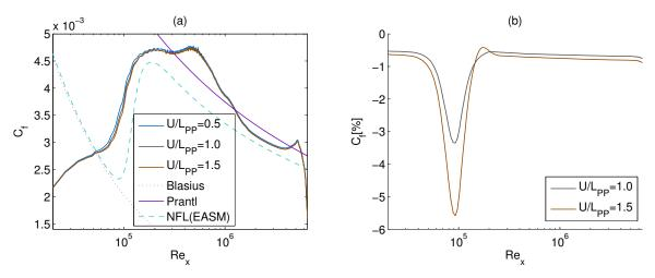
**Figure 9.** (a) Comparison of the local frictional resistance coefficients of H1 hull for the domain size variation in  $U/L_{PP}$  and (b) comparison of  $C_f$  of H1 hull relative to  $U/L_{PP} = 1$ .
