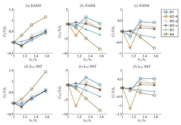
**Figure 2.** Computed values for (a)  $C_F$ , (b)  $C_{PV}$  and (c)  $C_V$  with the EASM model and (d)  $C_F$ , (e)  $C_{PV}$  and (f)  $C_V$  with the  $k - \omega$  SST model vs. grid refinement ratio,  $h_1/h_i = \sqrt[3]{N_{grid_1}/N_{grid_i}}$ .
