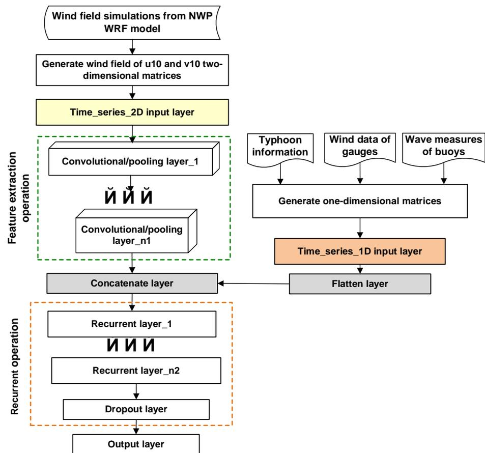
Figure 2. Architecture of an NUM–AI-based prediction model constructed with convolutional and recurrent neural networks and using numerical weather model outcomes.
