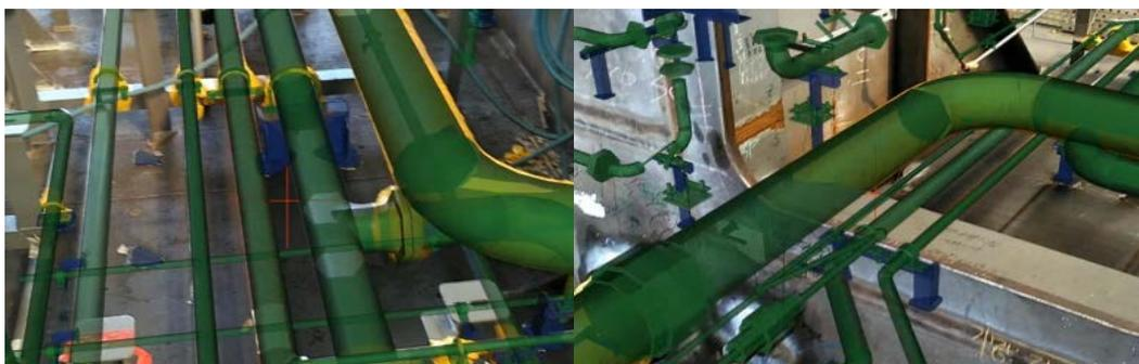
**Figure 15.** Examples of accurate AR scene generation. The pipe and pipe support CAD models are augmented very precisely on the real objects.
