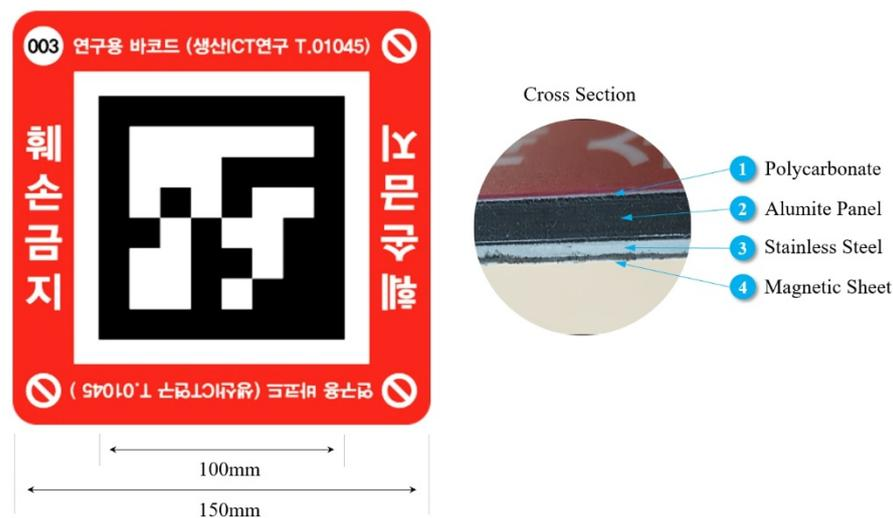
Figure 7. Design details of proposed marker.
