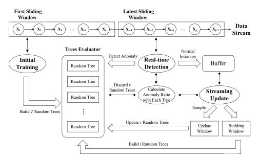
Figure 1. The workflow of unsupervised incremental anomaly detection.
