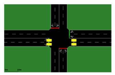
Figure 11. Arterial junction with sensor locations (yellow rectangle).
