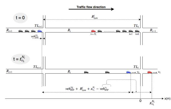
Figure 7. Illustration of adjacent traffic lights synchronization mechanism.
