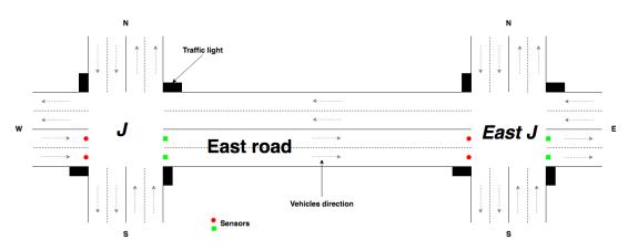
Figure 3. Illustration of sensors deployment on adjacent arterial junctions.
