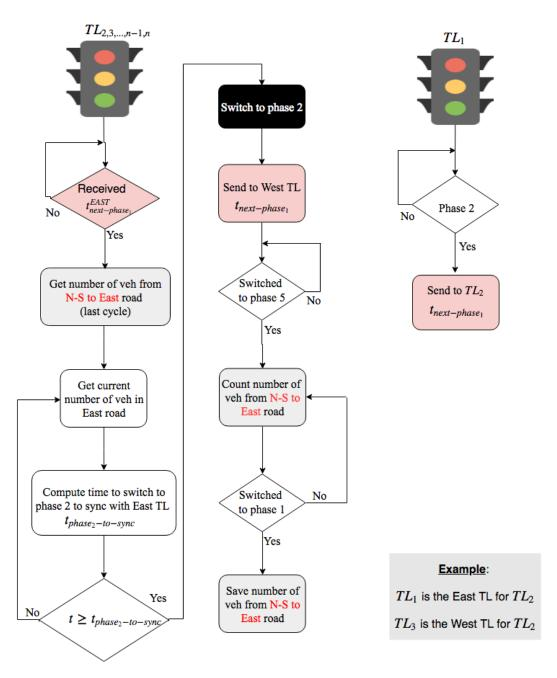
Figure 9. Illustration of TLs synchronization steps.
