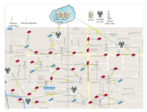
Figure 1. Vehicular navigation architecture.
