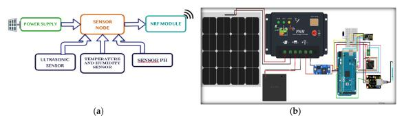
Figure 2. Structure of the Sensor Node (NS): (a) NS block diagram. (b) NS connection diagram.
