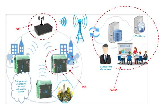
channel. The prototype design consists of three main parts, as shown in Figure 1: Sensor Node (NS), Gateway Node (NG), and Storage and Monitoring Node (NAM), which will be described in detail later.
