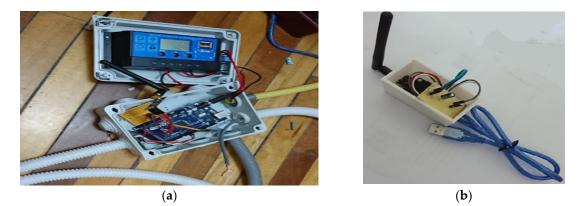
Figure 11. Implementation of Nodes: (a) Sensor Node. (b) Gateway Node.
