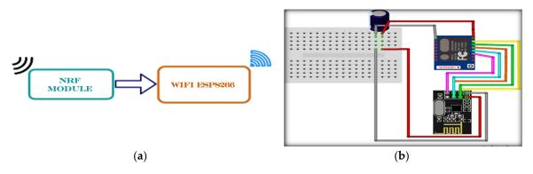
Figure 3. Structure of the gateway node (NG): (a) NG block diagram. (b) NG connection diagram.
