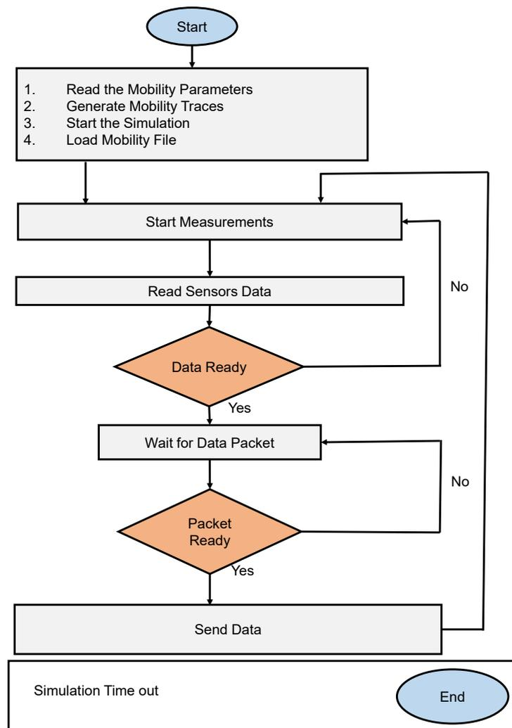
Figure 5. Simulation Flowchart.
