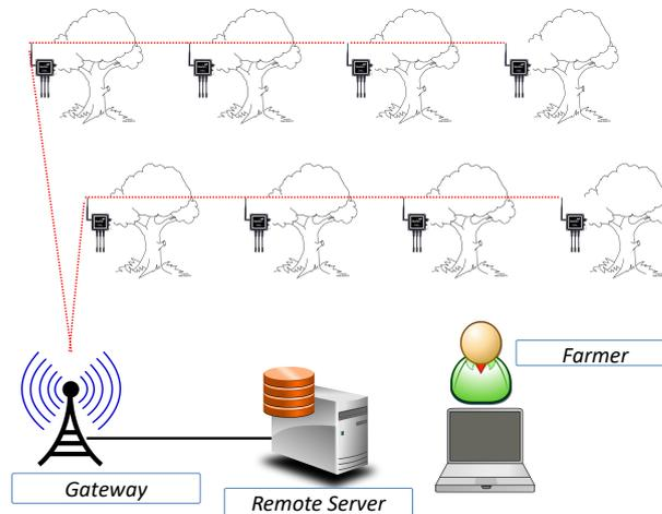
Figure 3. IoT system for monitoring olive trees in a fixed position.
