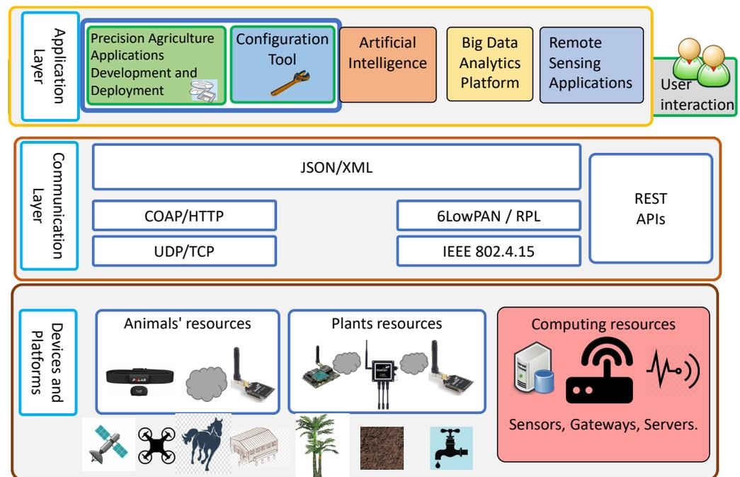
**Figure 1.** Proposed IoT system model for precision agriculture, showing the relationship between various entities such as sensors, network-enabling technologies, and agricultural resources for real-time monitoring and control.
