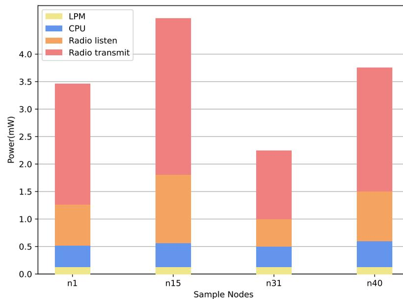
**Figure 9.** Instantaneous Power Consumption for nodes = [1, 15, 31, 40].
