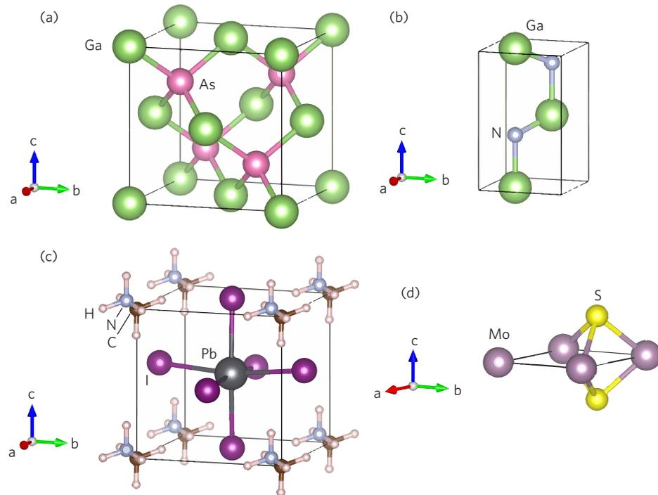
**Figure 1.** Crystal structures: (a) GaAs, (b) GaN, (c) quasi-cubic (CH<sub>3</sub>NH<sub>3</sub>)PbI<sub>3</sub>, and (d) mono-layer MoS<sub>2</sub>.
