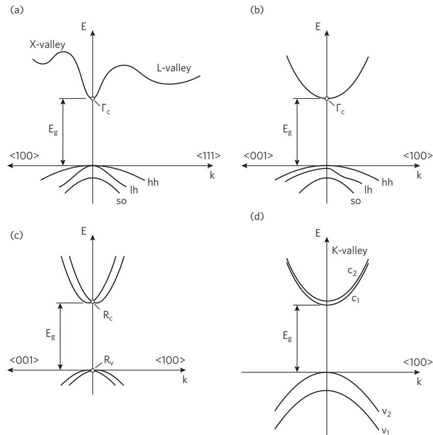
**Figure 2.** Schematic band structures of materials studied with SOC: (a) GaAs, (b) GaN, (c) quasi-cubic  $(CH_3NH_3)PbI_3$ , and (d) monolayer  $MoS_2$ . The band indices ‘c’, ‘hh’, ‘lh’, and ‘so’ stand for conduction, valence heavy-hole, light-hole, and split-off bands, respectively. The scale of band splittings is exaggerated.
