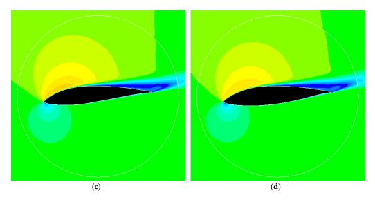
**Figure 13.** Predicted distribution of dimensionless velocity magnitude around the airfoil for Re = 100,000, BA = 5°, FA = 15° (AoA = 10°), for L/C = 6, (**a**) Original profile; (**b**) Point 1; (**c**) Point 2; (**d**) Point 3 (Figure 9).
