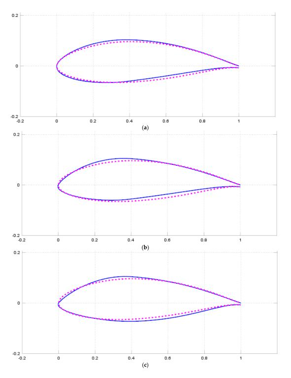
**Figure 10.** Optimized airfoil shapes for L/C = 3, for the points indicated by full arrows in Figure 9 (a) Point 1; (b) Point 2; (c) Point 3 (Figure 8), red dotted line: original, blue solid line: optimized (note that vertical scale is larger than horizontal scale).
