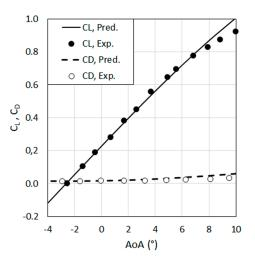
**Figure 6.** Comparison of predicted lift and drag coefficients with the measured values for the profile NREL-S822 of Selig et al. [51] (Re = 400,000).
