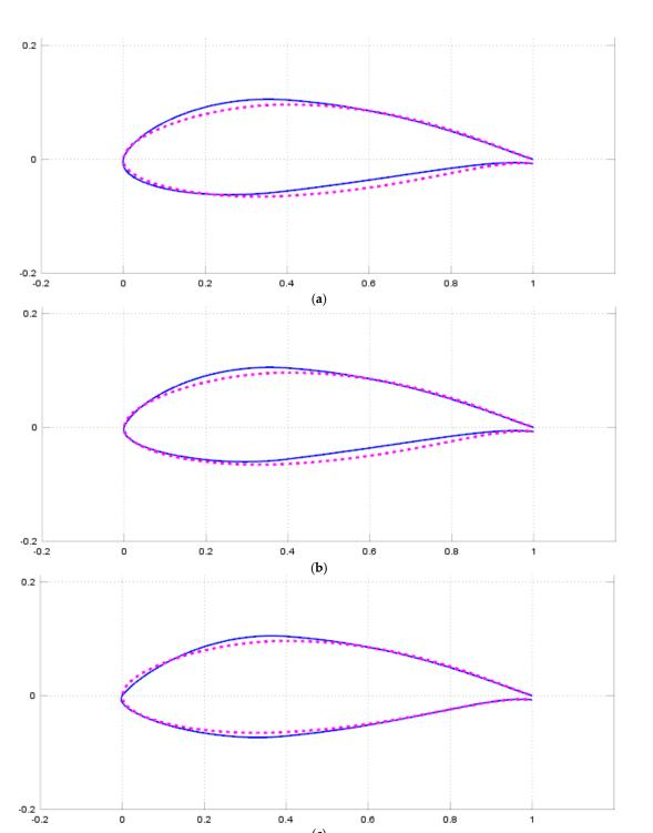
**Figure 11.** Optimized airfoil shapes for L/C = 6, for the points indicated by empty arrows in Figure 9 (a) Point 1; (b) Point 2; (c) Point 3 (Figure 8), red dotted line: original, blue solid line: optimized (note that vertical scale is larger than horizontal scale).
