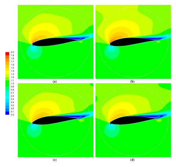
**Figure 12.** Predicted distribution of dimensionless velocity magnitude around the airfoil for Re = 100,000, BA = 5°, FA = 15° (AoA = 10°), for L/C = 3, (a) Original profile; (b) Point 1; (c) Point 2; (d) Point 3 (Figure 9).
