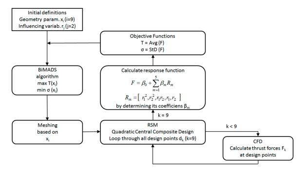
Figure 8. Detailed representation of the optimization cycle.
