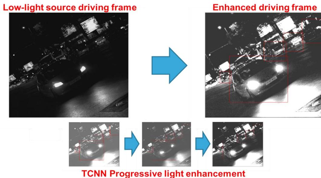
**Figure 7.** A detail of the enhanced low-light driving frames with embedding bounding-box (red box) and light-processing performed by the proposed TCNN as per Equations (5)–(7).
