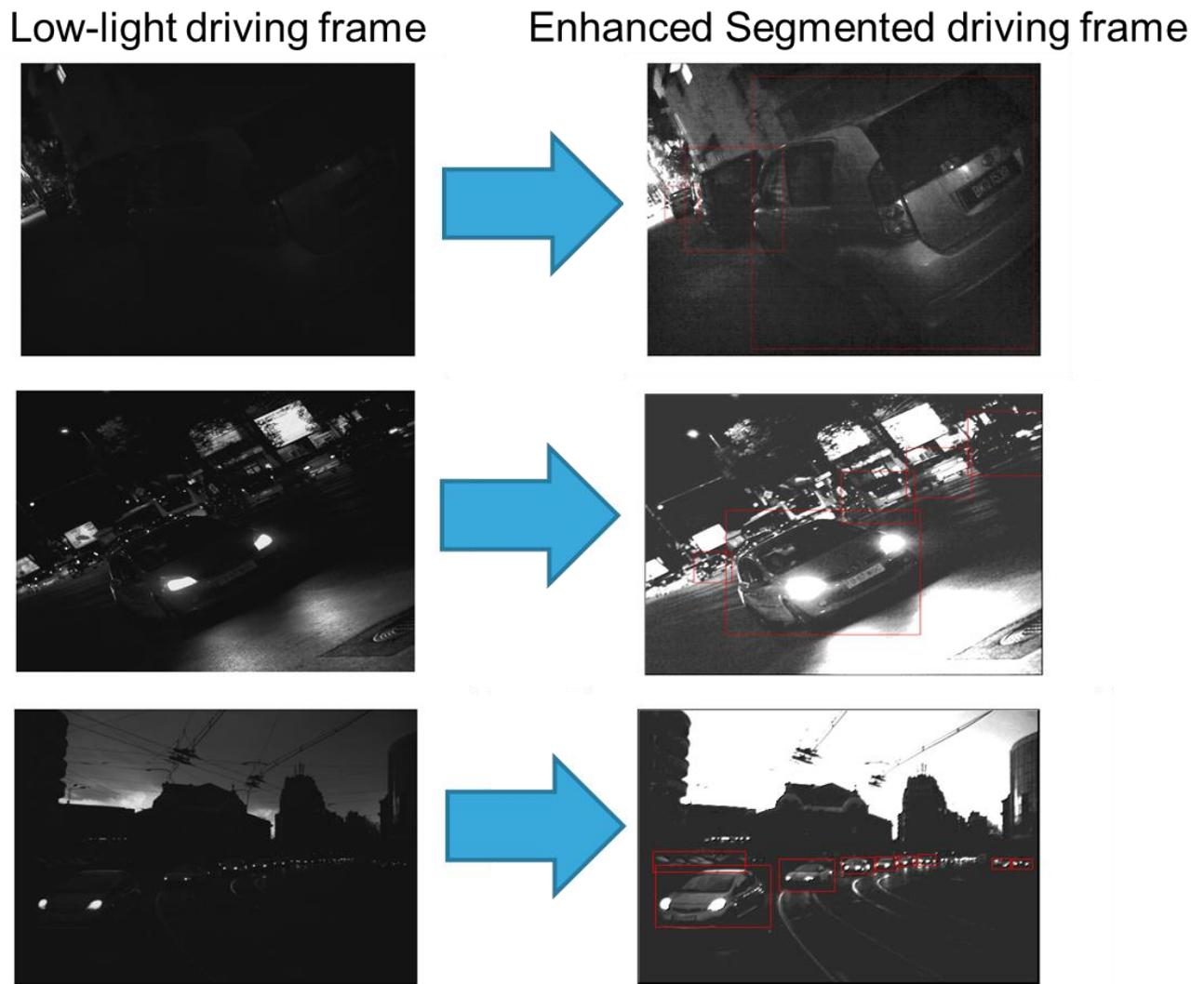
Figure 6. Some instances of the low-light driving frames with corresponding enhanced and segmented frames.
