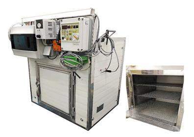
Figure 1. Laboratory-scale convective dyer and three-perforated tray drying chamber.
