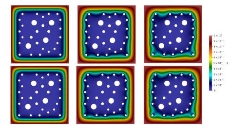
**Figure A1.** Parabolic problem with  $\alpha = 100$  for different time layers  $t_m$  with m = 5, 15, and 40 (from **left** to **right**). Case 1 (homogeneous boundary conditions). **Top**: Reference solution ( $DOF_h = 85,230$ ). **Bottom**: Multiscale solution with 12 multiscale basis functions,  $e_{L^2} = 2.22$  for  $t_1$ ,  $e_{L^2} = 1.605$  for  $t_{10}$ ,  $e_{L^2} = 1.058$  for  $t_{40}$  ( $M_g = M = 12$ ,  $M_p = 0$ ,  $DOF_H = 1300$ ).
