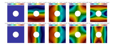
**Figure 4.** Illustration of the outer boundary multiscale basis functions for elasticity problem,  $\psi_{g,k}^{l}$  for k = 1, ..., 5 (from **left** to **right**). First row: displacement X-component. Second row: displacement Y-component.
