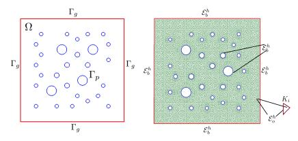
**Figure 1.** Illustration of perforated domain  $\Omega$  (**left**) and fine grid  $\mathcal{T}^h$  (**right**).
