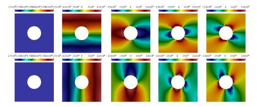
**Figure 6.** Illustration of the perforation boundary multiscale basis functions for elasticity problem,  $\psi_{p,k}^{i}$  for k = 1, ..., 5 (from **left** to **right**). First row: displacement X - component. Second row: displacement Y-component.
