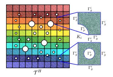
**Figure 2.** Coarse grid  $\mathcal{T}^H$  with coarse cell  $K_i$ ,  $\Gamma_g^i \cup \Gamma_p^i = \partial K_i$ .
