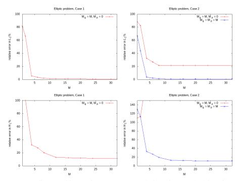
**Figure 8.** Elliptic problem with  $\alpha = 100$ . Case 1 (left) and Case 2 (right): Relative  $L_2(top)$  and  $H_1(bottom)$  error with a different number of multiscale basis functions.
