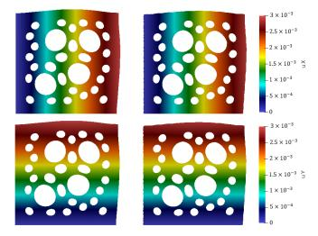
**Figure 11.** Elasticity problem. Case 1 (homogeneous boundary conditions). First row: displacement X-component. **Left:** Reference solution ( $DOF_h = 170,460$ ). **Right:** Multiscale solution with 24 multiscale basis functions,  $e_{L^2} = 2.117$  ( $M_g = M = 24$ ,  $M_p = 0$ ,  $DOF_H = 4900$ ).
