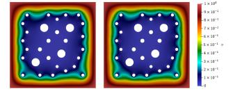
**Figure 9.** Elliptic problem with  $\alpha = 100$ . Case 1 (homogeneous boundary conditions). **Left**: Reference solution ( $DOF_h = 85,230$ ). **Right**: Multiscale solution with 12 multiscale basis functions,  $e_{L^2} = 1.053$  ( $M_g = M = 12$ ,  $M_p = 0$ ,  $DOF_H = 1300$ ).
