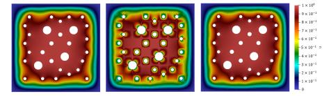
**Figure 10.** Elliptic problem with  $\alpha = 100$ . Case 2 (non-homogeneous boundary conditions). **Left**: Reference solution ( $DOF_h = 85,230$ ). **Center**: Multiscale solution with 12 multiscale basis functions without perforation basis functions,  $e_{L^2} = 21.52$  ( $M_g = M = 12$ ,  $M_p = 0$ ,  $DOF_H = 1300$ ). **Right**: Multiscale solution with 12 multiscale basis functions with perforation basis functions,  $e_{L^2} = 0.772$  ( $M_g = M_p = M = 12$ ,  $DOF_H = 1776$ ).
