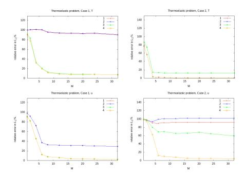
**Figure A4.** Thermoelasticity problem. Temperature (**top**) and Displacement (**bottom**). Case 1 and Case 2: Relative  $L_2$  error with a different number of multiscale basis functions. (1)  $M_g^u = M^u$ ,  $M_p^u = 0$  and  $M_g^T = M^T$ ,  $M_p^T = 0$ ; (2)  $M_g^u = M^u$ ,  $M_p^u = 0$ , and  $M_g^T = M_p^T = M^T$ ; (3)  $M_g^u = M_p^u = M^u$  and  $M_g^T = M^T$ ,  $M_p^T = 0$ ; (4)  $M_g^u = M_p^u = M^u$  and  $M_g^T = M_p^T = M^T$ .
