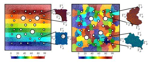
Figure 14. Coarse grids and local domains. (Left): quasi-structured grid. (Right): unstructured grid.
