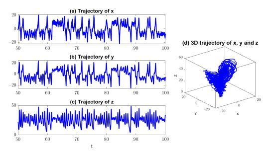
**Figure 1.** The noisy Lorenz 63 model (12) with parameters in (13). (**a**–**c**) one realization of the onedimensional trajectories of x, y, and z, respectively; (**d**) the associated three-dimensional phase plot of (x, y, z).
