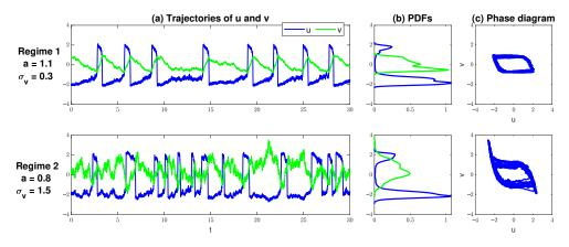
**Figure 4.** The two dynamical regimes of the stochastically coupled FHN model (14), where the parameters of the two regimes are listed in (15) and (16). The three columns show the model trajectories, the PDFs, and the phase diagram of both dynamical regimes.
