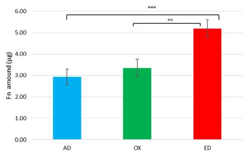
**Figure 1.** Surface protein quantities after 1% SDS rinses for the Fn initially adsorbed (AD), oxidized (OX), or electrodeposited (ED) on PPy-coated 316L SS supports. Values are means  $\pm$  standard error means. Data are representative of three independent experiments performed in triplicate; significant differences were determined using a one-way ANOVA analysis, and the *p*-value of the test is 0.0004 (\*\* p < 0.01, \*\*\* p < 0.001).
