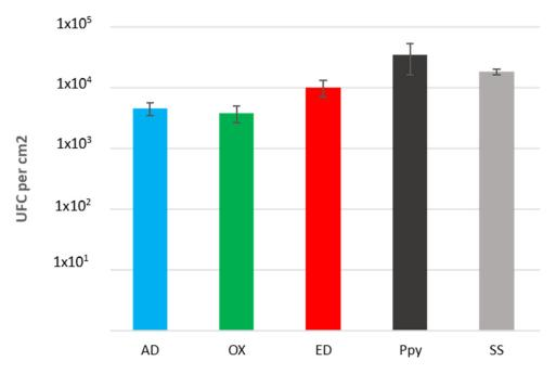
**Figure 8.** Bacterial attachment on bio-functionalized supports. Number of *Staphylococcus aureus* CIP4.83 bacteria adhering on Fn adsorbed (AD), oxidized (OX), electrodeposited (ED), polypyrrole (PPy) coating, or stainless steel (SS) substrate. The incubation time was 3 h. Values are means  $\pm$  standard error means (n = 2).
