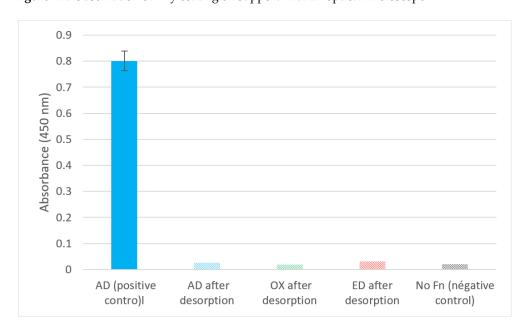
**Figure A2.** ELISA test of Fn adsorbed (AD), oxidized (OX), or electrodeposited (ED) on PPy-coated 316L SS substrates after desorption using a polyclonal antibody targeting Fn. Positive control was performed with Fn adsorbed (AD) without desorption, and negative control was performed with substrate without Fn coating.
