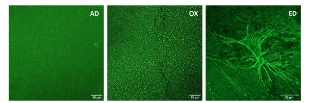
Figure 2. Images of Fn adsorbed (AD), oxidized (OX), or electrodeposited (ED) on PPy-coated 316L SS supports. Fn was immunostained to be observed by CSLM. Scale bar:  $50 \mu m$ . Data are representative of two different experiments.
