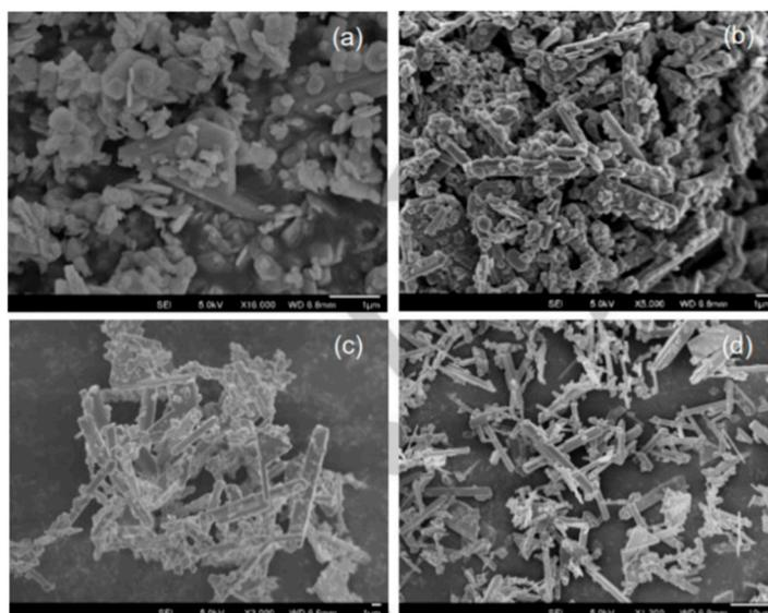
**Figure 3.** SEM images of  $\alpha$ -ZrP prepared by the minimal solvent synthesis method with  $F^-$  ions at different reaction times; (a) 1 h (b) 4 h (c) 8 h and (d) 96 h. Reproduced from [40], with permission from John Wiley and Sons, 2017.
