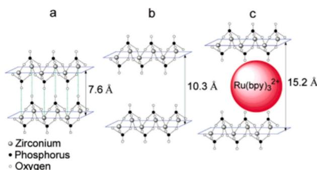
**Figure 6.** Schematic representation of (a)  $\alpha$ -ZrP (b)  $\theta$ -ZrP and (c)  $[\text{Ru}(\text{bpy})_3]^{2+}$ -exchanged ZrP. Reproduced from [13], with permission from the American Chemical Society, 2003.
