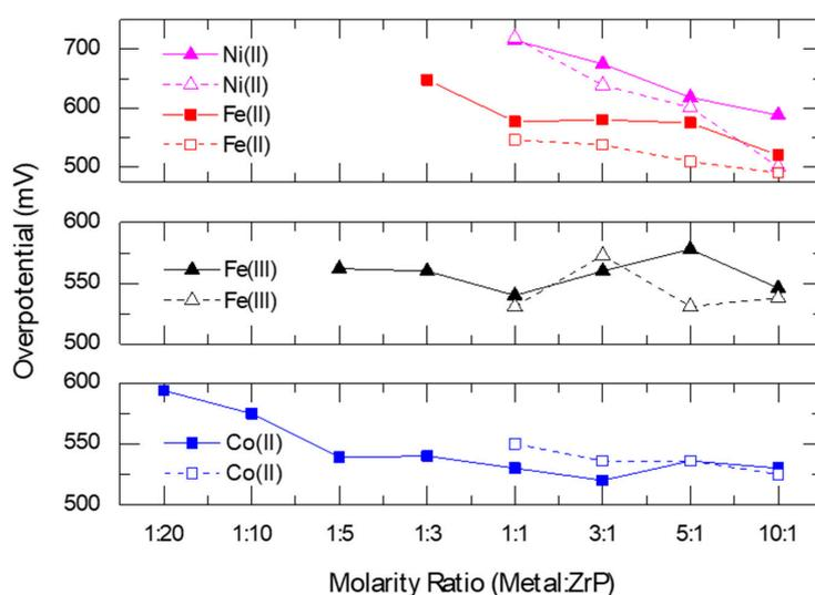
**Figure 9.** Overpotential as a function of M:ZrP synthesis ratio for the different metal-modified ZrP catalysts. Dashed lines correspond to surface-adsorbed catalysts while the solid line correspond to metal-intercalated catalysts. Taken from reference [87].
