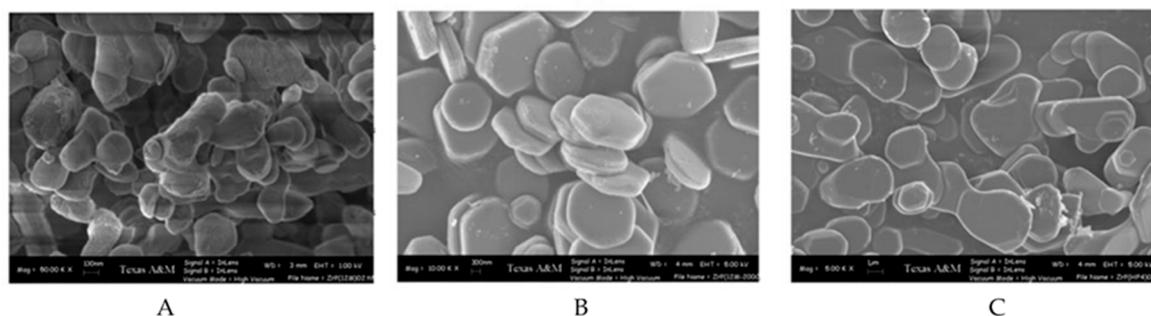
**Figure 2.** SEM images of  $\alpha$ -ZrP prepared by (A) reflux method (12 M  $\text{H}_3\text{PO}_4$ ) (B) hydrothermal method (9 M  $\text{H}_3\text{PO}_4$ ) (C) HF method (F/Zr = 4). [34]—Adapted by permission of The Royal Society of Chemistry on behalf of the Centre National de la Recherche Scientifique, 2007.
